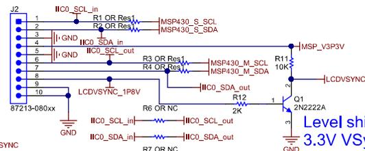
Level shifter from 1.8V to 3.3V VSync from DLPC343x
