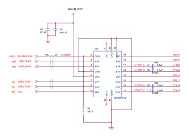
Port select pin (SEL). Internally tied to GND via 100k resistor. L: Port A to Port B H: Port A to Port C
