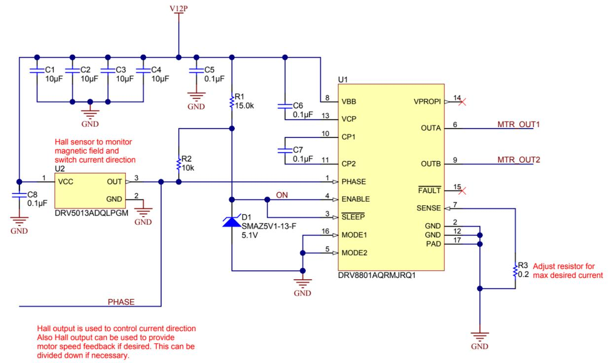
Hall sensor to monitor magnetic field and switch current direction
