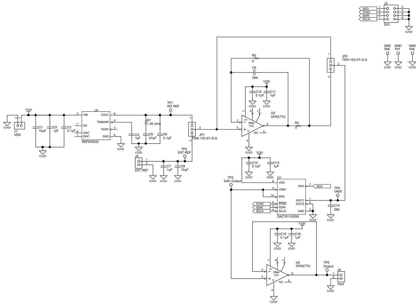
TIPD159: Voltage-Mode Multiplying DAC Reference Design
