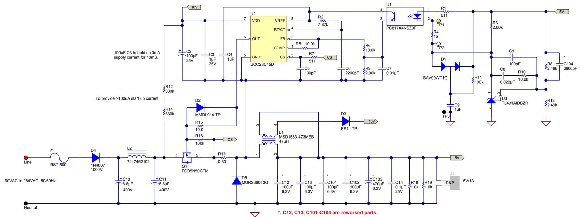
100uF C3 to hold up 3mA supply current for 10mS.
