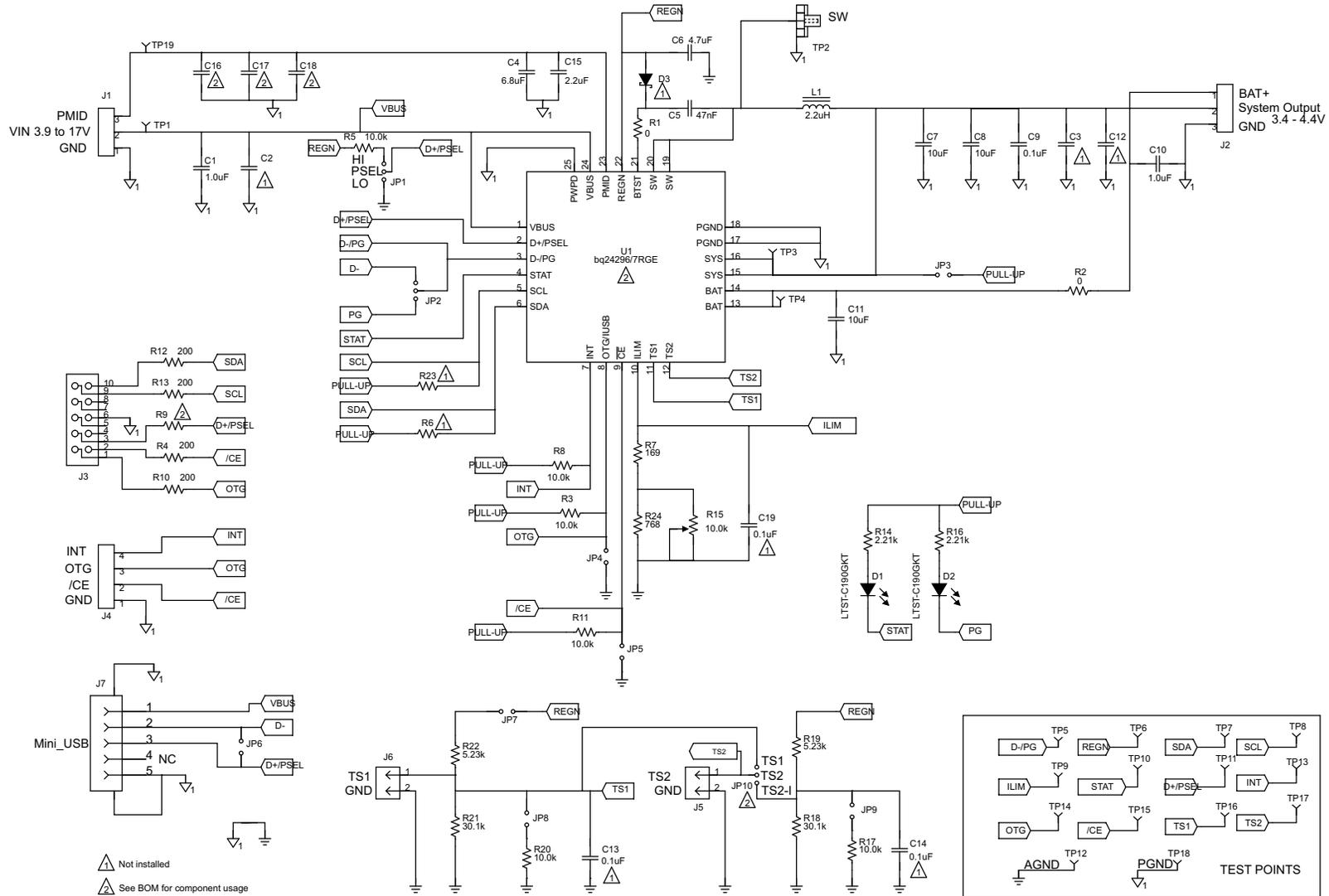
Figure 12. bq24x9xEVM Schematic
