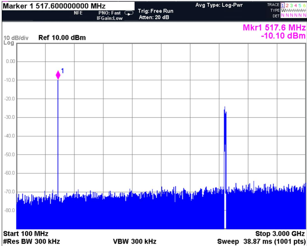
Figure 7 shows the dither at the TX output in addition to the desired signal. However, the frequency response of the signal path following the DAC will prevent this from appearing at the antenna output.
