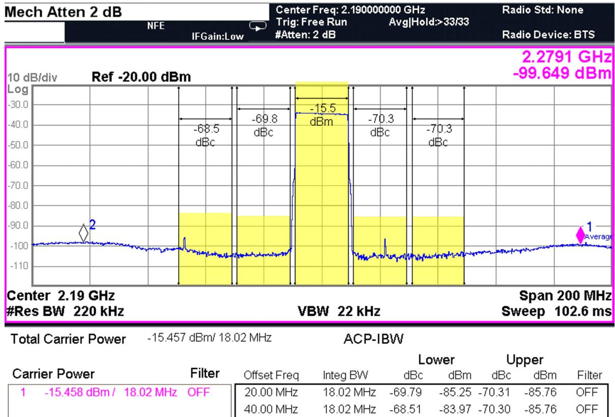
The ACPR improved by as much as 8 dB with the use of dither. Markers 1 and 2, respectively, show HD3 and HD5 with levels around -100 dBm.
