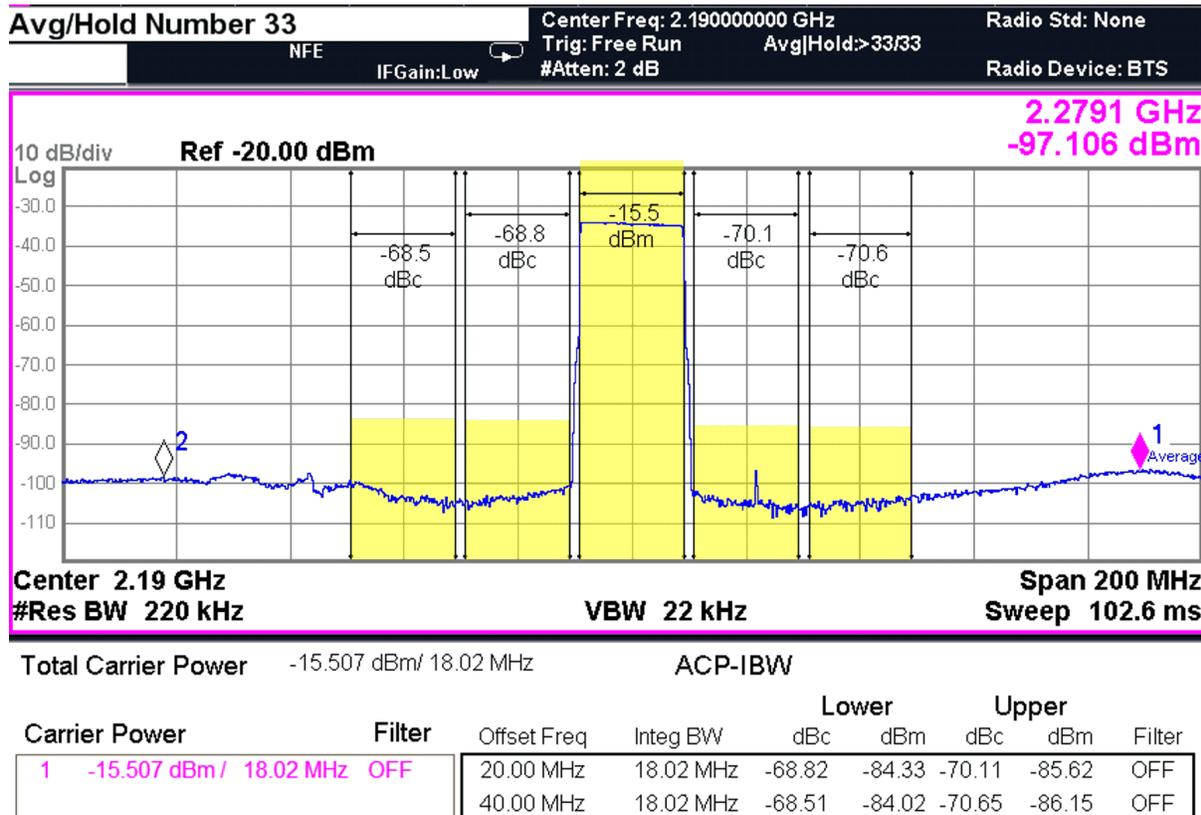
Figure 5 shows the TX output with lower dither level (-21 dB instead of -6 dB) and the divide-by-2 enabled to avoid saturation. The channel power is now 6 dB lower and leakage performance improved. The  $F_{DAC} / 4$  spur in the upper adjacent channel is low enough to meet the unwanted emissions specification.
