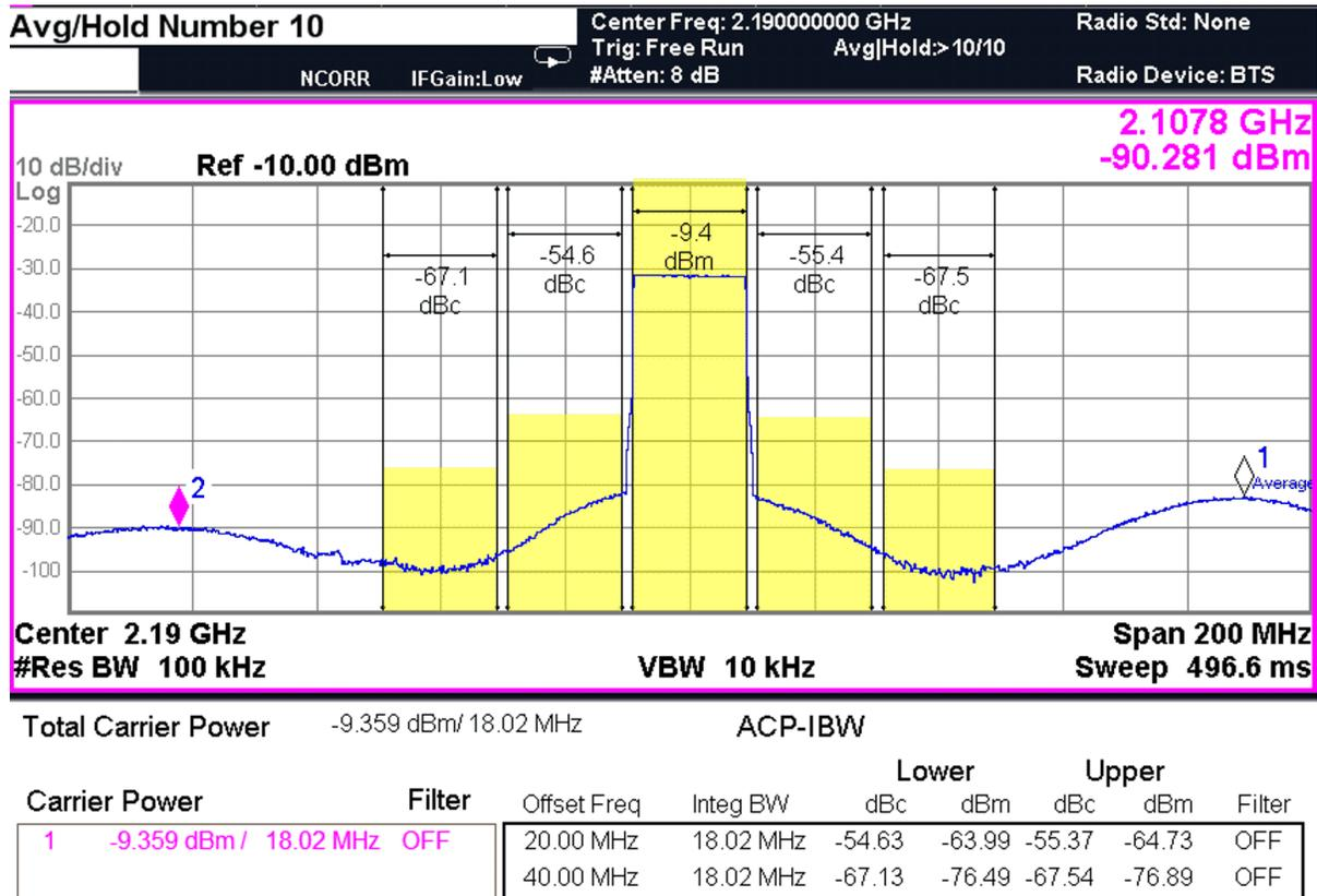
Figure 4 shows a dither setting (0x32=0x6, 0x33=0x2) with the divide-by-2 disabled with signal input at full-scale. The DAC starts to saturate (due to the full-scale input and large dither level) resulting in degraded spectrum. The fix is to enable the divide-by-2 to prevent clipping (0x33<3>=0x1).
