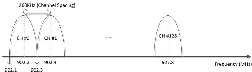
Figure 1. PHY ID #1 (FCC Band: 902 MHz to 928 MHz)
