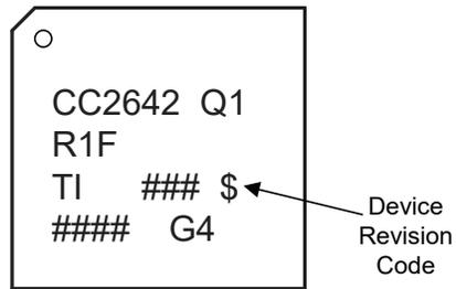
**Figure 2-1. Package Symbolization for Silicon Revision E**
