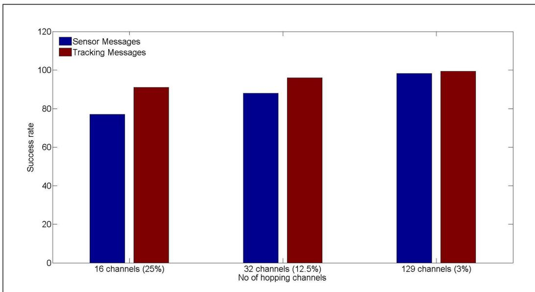
**Figure 5:** Robustness across increased number of hopping channels
