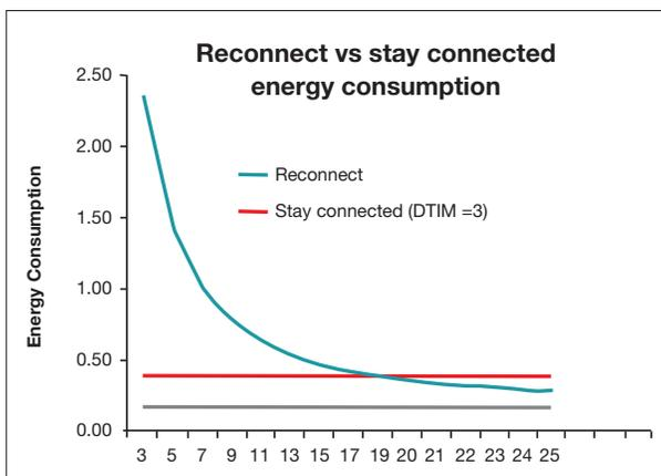
**Figure 5.** Reconnect vs. stay connected application energy consumption
