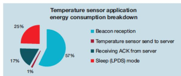
**Figure 4.** Temperature sensor application energy consumption breakdown
