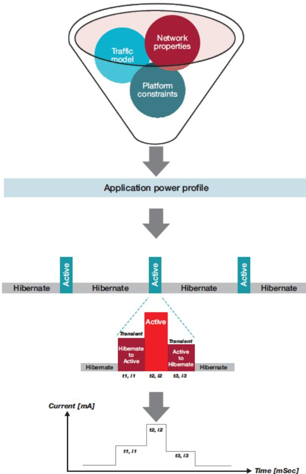
**Figure 2.** Application energy consumption profile analysis flow
