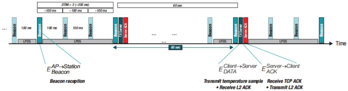
**Figure 3.** Temperature sensor power profiles and system modes
