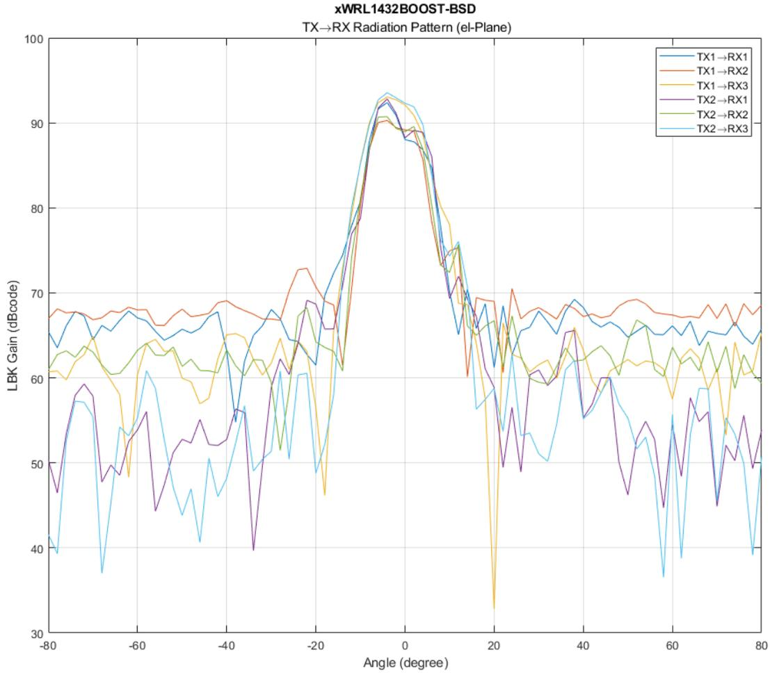
**Figure 2-8. xWRL1432BOOST-BSD EVM Antenna Elevational Radiation Pattern**
