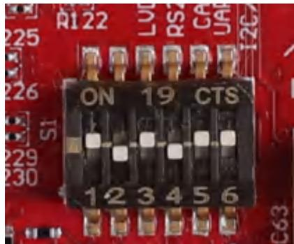
Figure 2-10. S1 Switch for Various Mode Settings
