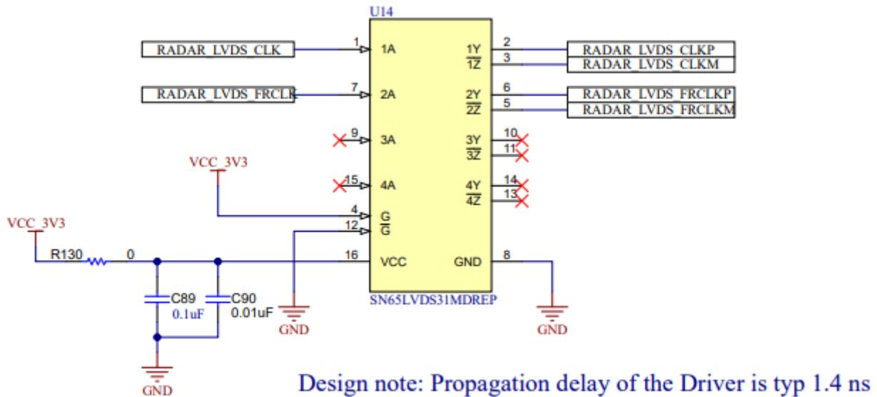
**Figure 2-26. DCA1000 CMOS TO LVDS Conversation for Clock and Control Lines**
