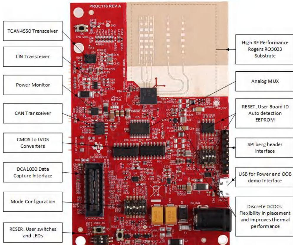
**Figure 2-3. Salient Features of EVM (Top Side)**
