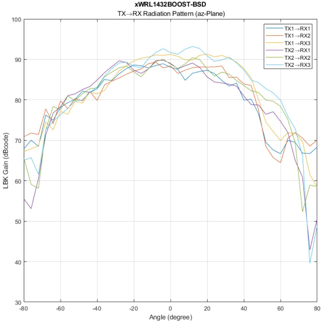
**Figure 2-7. xWRL1432BOOST-BSD EVM Antenna Azithmal Radiation Pattern**
