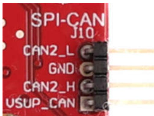
Figure 2-16. SPI-CAN Connector
