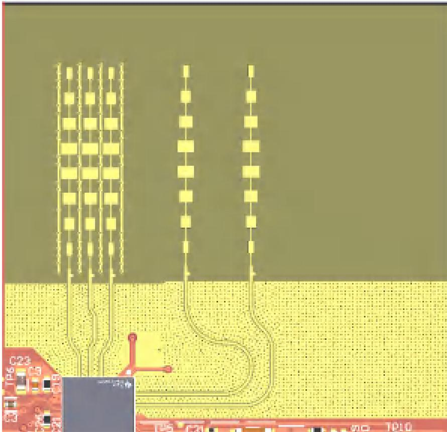
**Figure 2-5. TX and Rx Antennas of the EVM**
