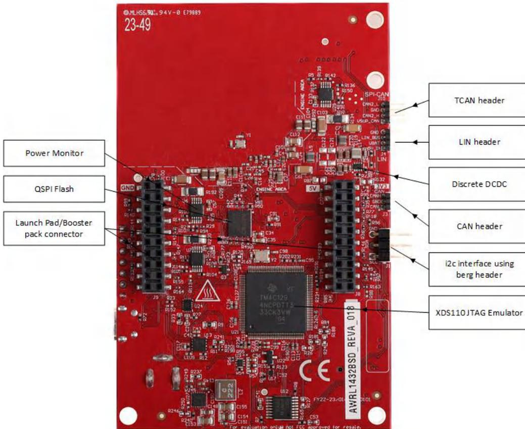
Figure 2-4. Salient Features of EVM (Bottom Side)
