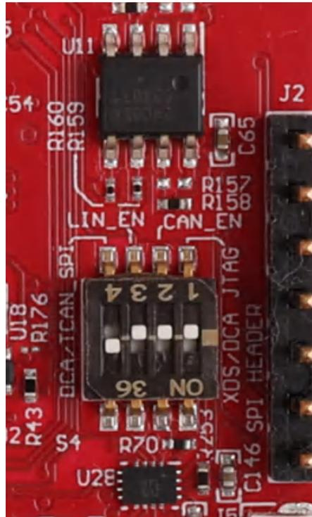
**Figure 2-11. S4 Switch for Various Mode Settings**
