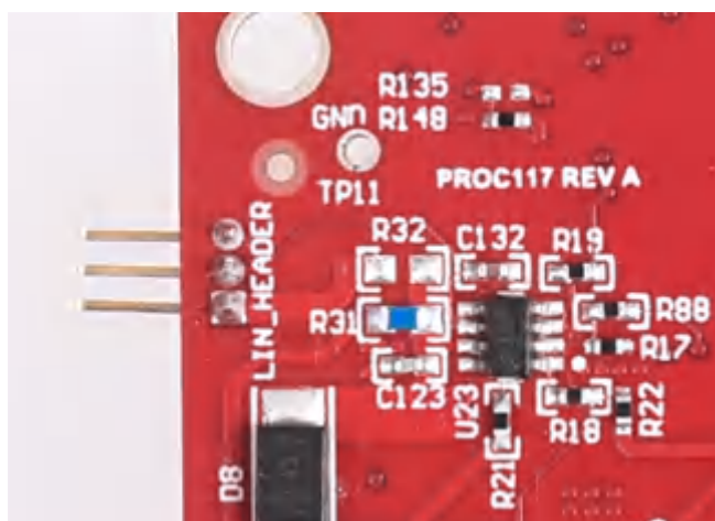
Figure 6-14. LIN header and PHY interface
