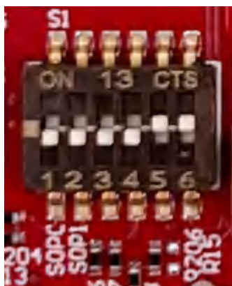
Figure 6-5. S1 Switch for Various Mode Settings
