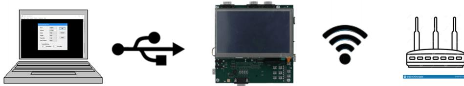
**Figure 9-1. Wi-Fi Station Hardware Setup**
