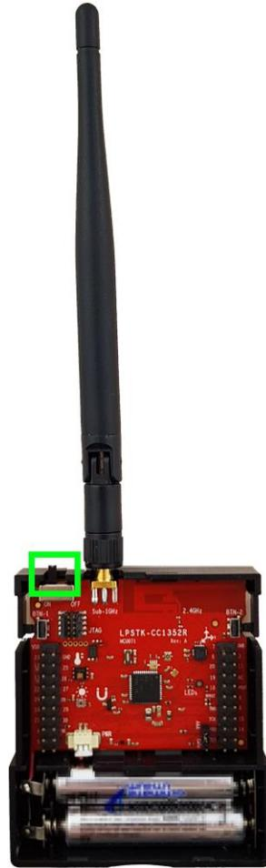
5. Add the CC1352R LaunchPad SensorTag as a new MIOTY end-point device in gateway with the following parameters:
