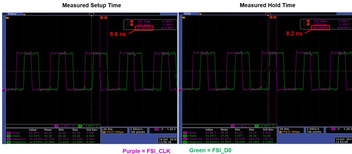
**Figure 12. RS485 - FSIRX Setup and Hold Time Measurements**
