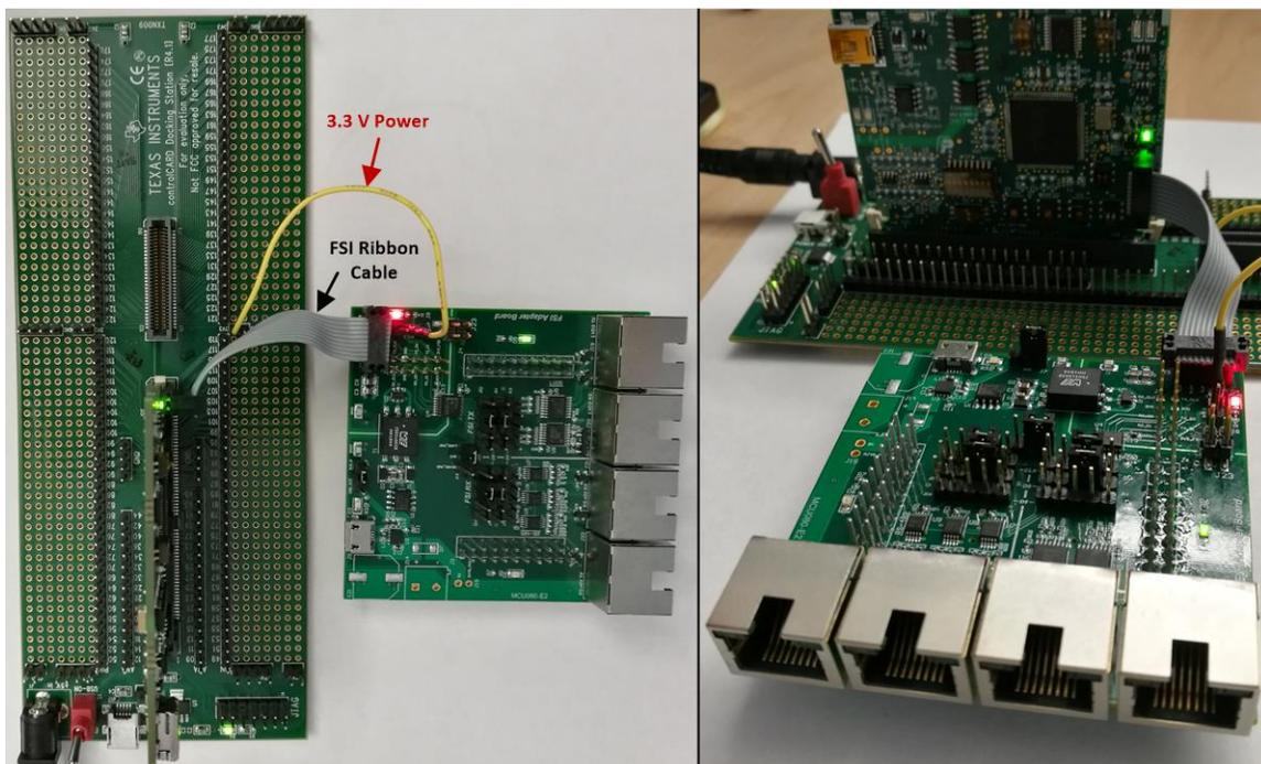
**Figure 6. controlCARD Setup**
