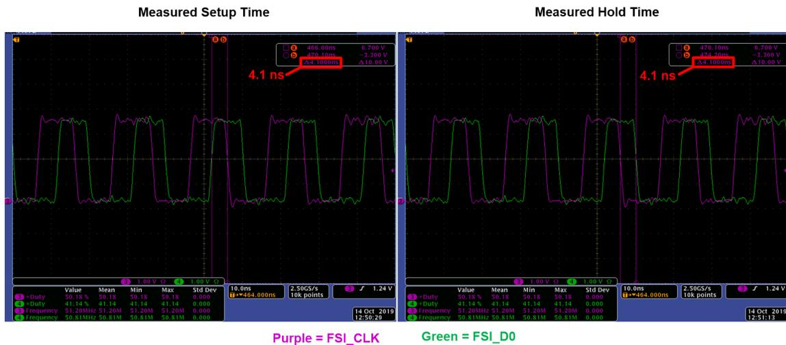
Figure 11. LVDS - FSIRX Setup and Hold Time Measurements
