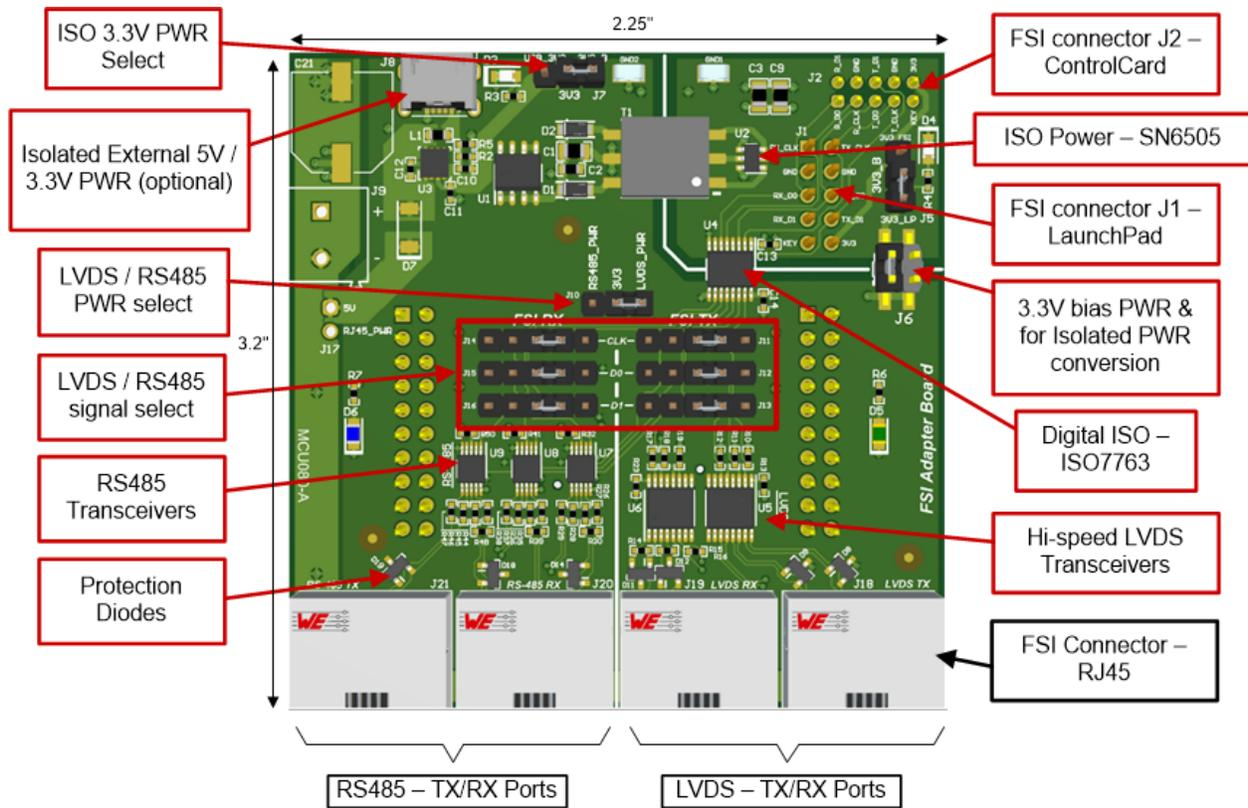
Figure 2. FSI Adapter Board - Front Side Hardware
