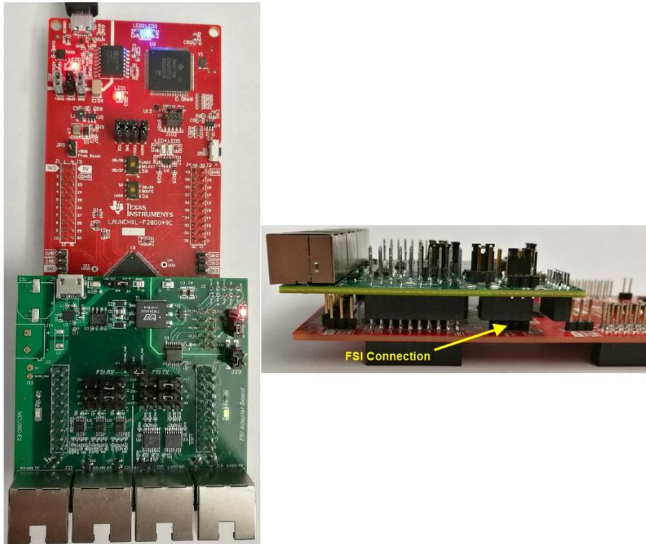
**Figure 4. LaunchPad Setup**
