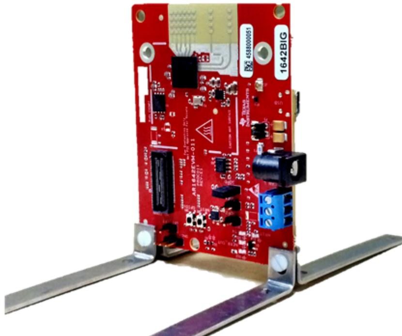
**Figure 22. Vertical Assembly of EVM**
