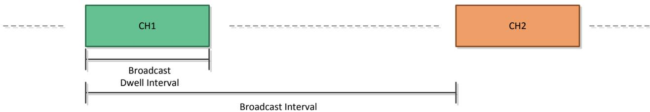
**Figure 4-17. Broadcast Channel Hopping Sequence**
