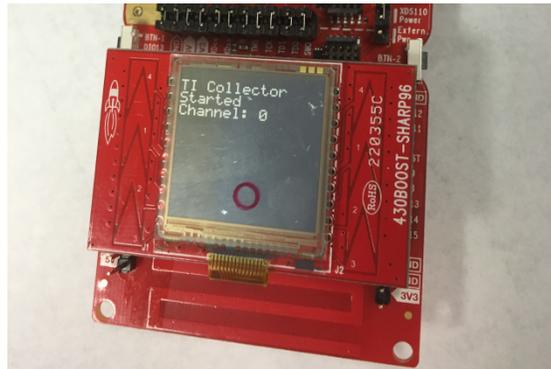
**Figure 6-4. LCD Display (1 of 2)**
