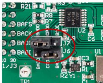
If audio is unused, the pins can be disabled from the connector to provide extra analog pins. Perform the following steps to disable the audio pins:
