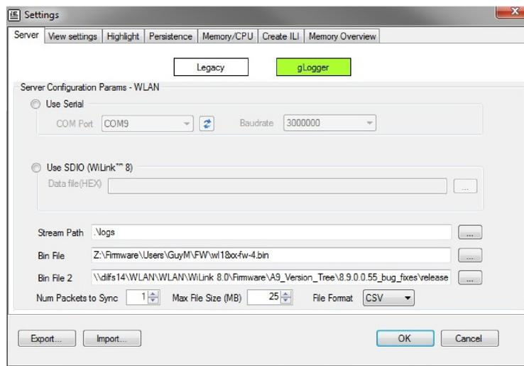
**Figure 3. Configuring the gLogger for UART Mode**
