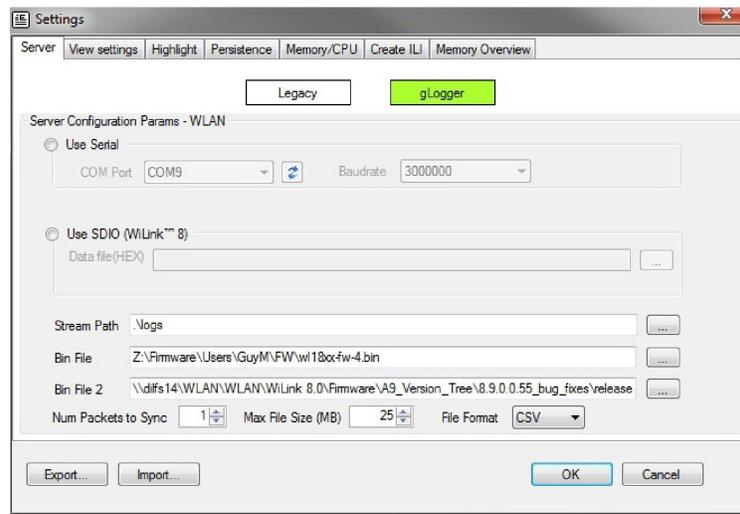
**Figure 4. Configuring the Logger for SDIO Mode**
