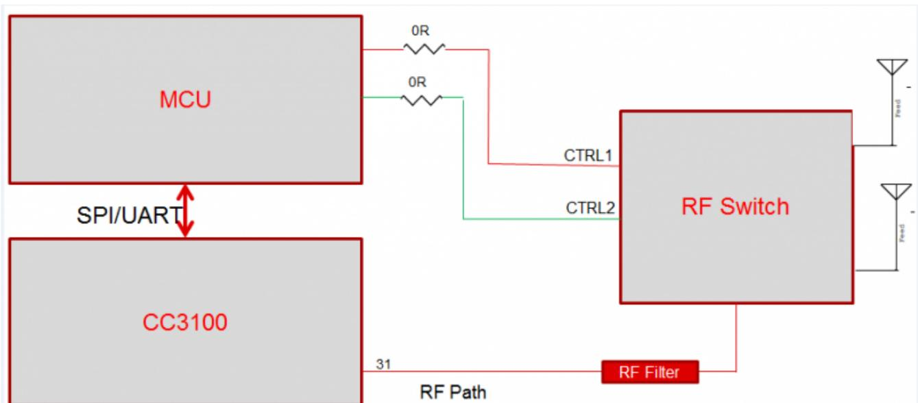
Figure 4-3. Diagram of the Boards' Connections
