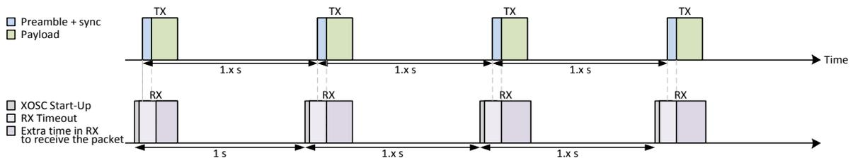
**Figure 30: eWOR Mode (RX and TX re-synchronized)**
