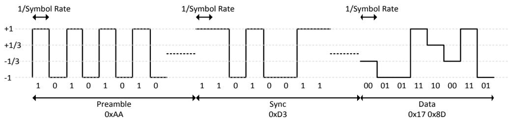
**Figure 9: Data Sent Over the Air (`CFM_DATA_CFG.SYMBOL_MAP_CFG = 0`)**
