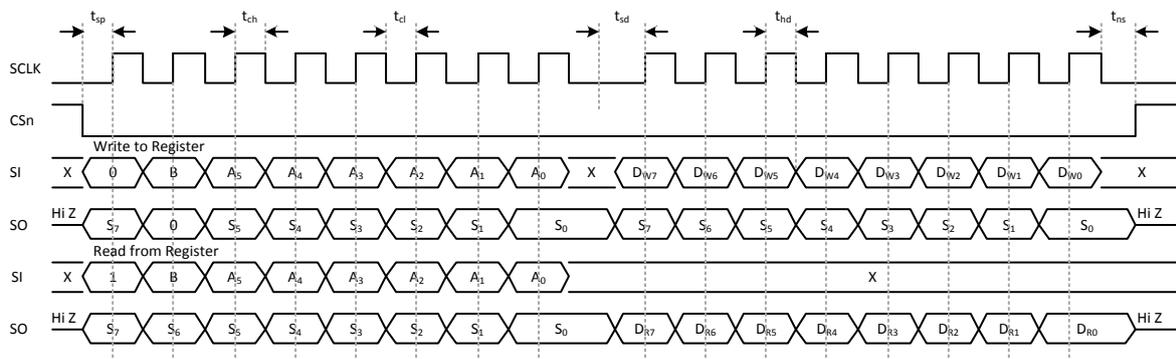
**Figure 3: Configuration Registers Write and Read Operations**
