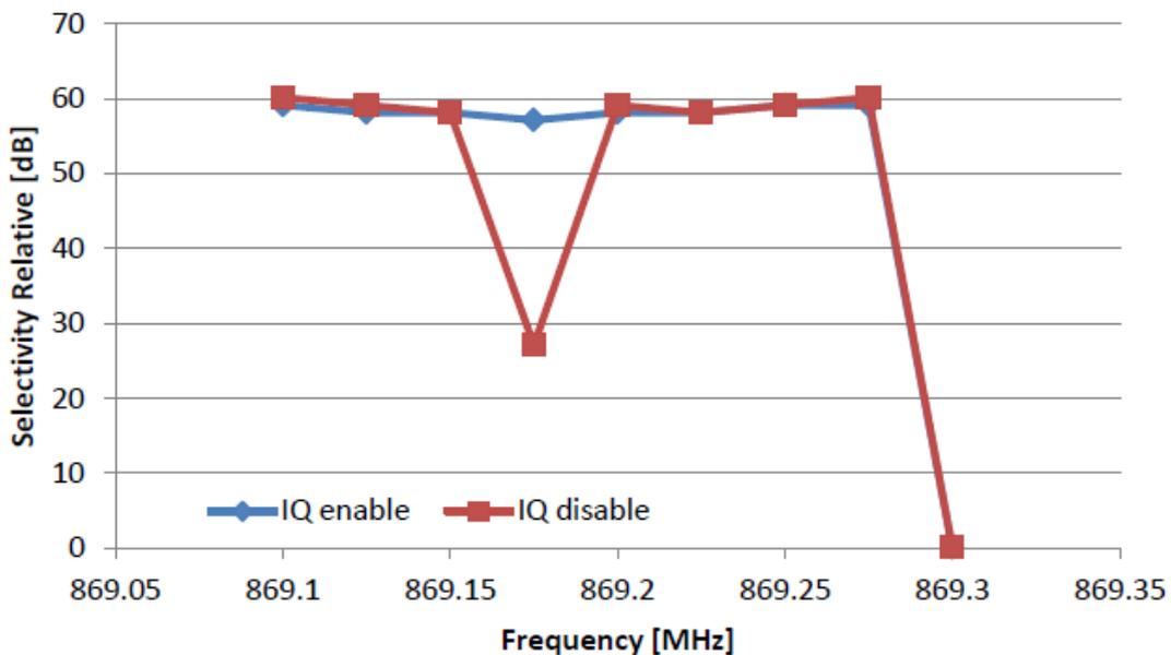
Figure 14: IQIC Enabled/Disabled (image at -125 kHz offset)
