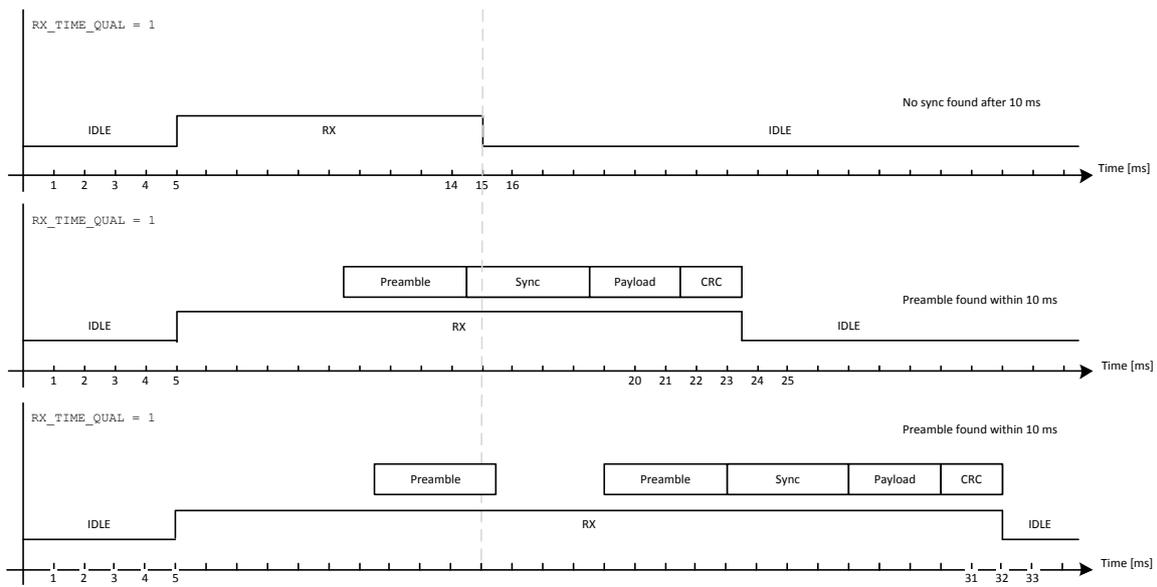
**Figure 25: RX Termination when `RX_TIME_QUAL = 1` (RX Timeout = 10 ms)**
