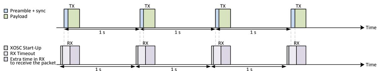
**Figure 28: eWOR Mode (RX and TX in sync.)**
