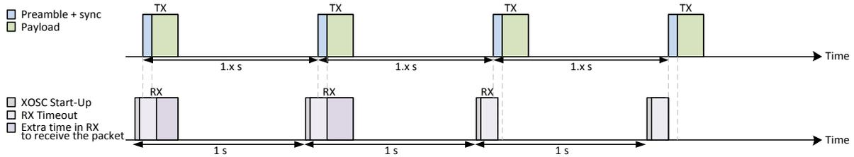
**Figure 29: eWOR Mode (RX and TX out of sync.)**
