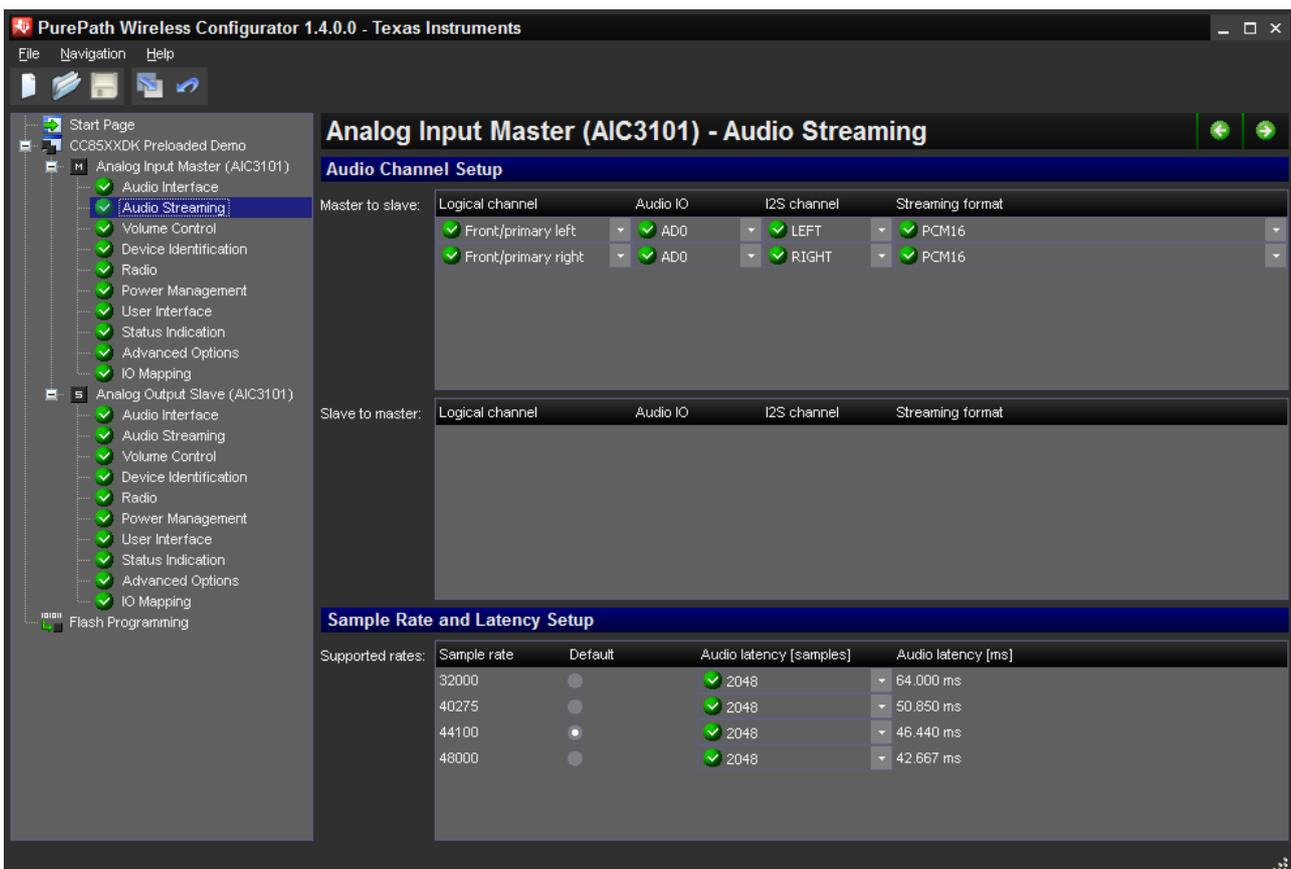
Figure 5 - PurePath Wireless Configurator screenshot
