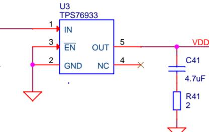
DC-DC for low loss 3.33V LED voltage supply
