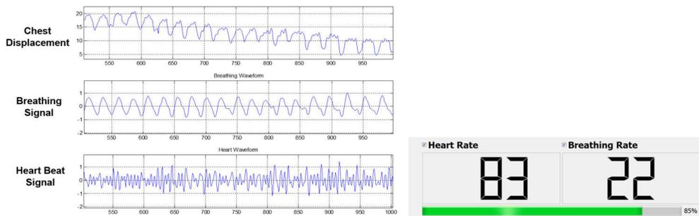
**Figure 3. Chest Movement Detected by mmWave Sensor; Separate Chest Movement Into Heart Beat Signal and Breathing Signal**
