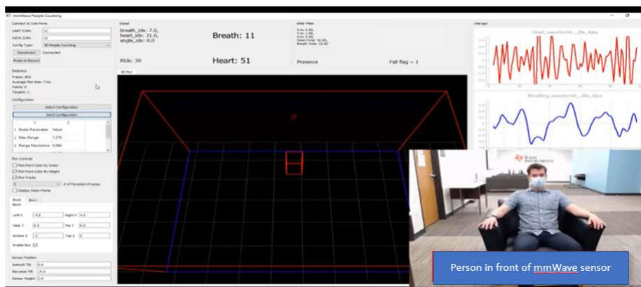
**Figure 4. Demonstration Of Vital Sign Detection Using IWR6843 Device From Texas Instruments**
