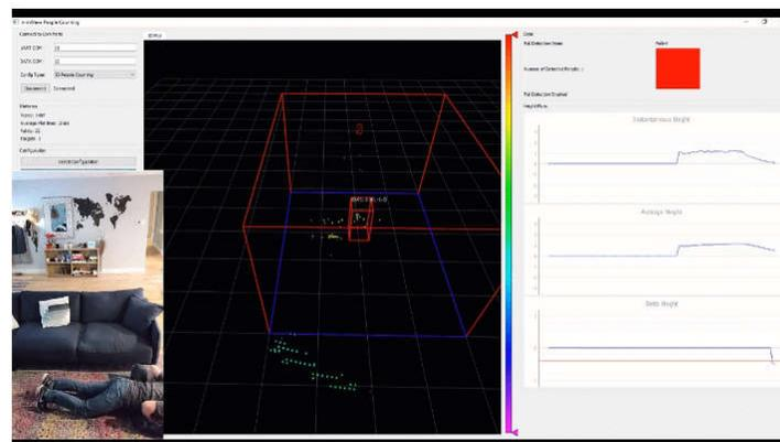
**Figure 2. Detection of the Fall Event of a Person Using IWR6843 Radar**
