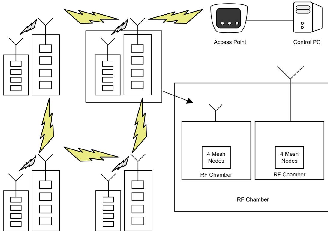
**Figure 11-2. WiLink™ 8 32 Mesh Nodes Test Setup Illustration**
