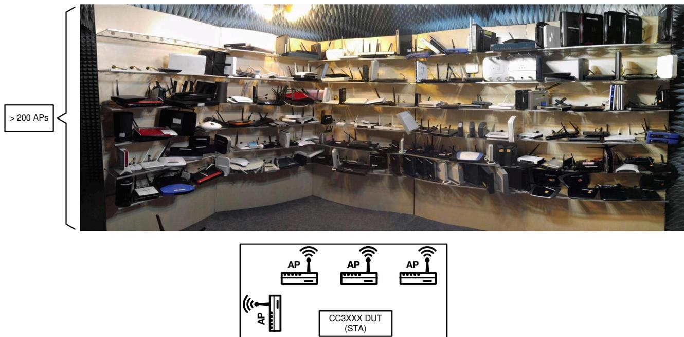
**Figure 2-1. IOP Chamber with Over 230+ AP Deployed Worldwide**
