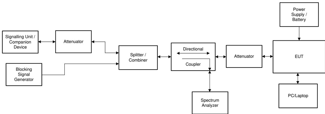
**Figure 3-2. Test Setup for Receiver Blocking – EN 300 328**
