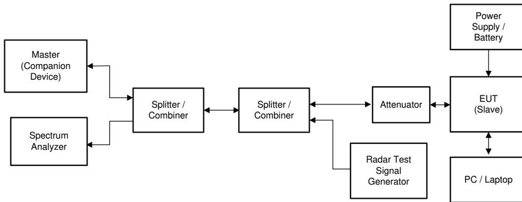
**Figure 4-3. Test Setup for DFS – EN 301 893**
