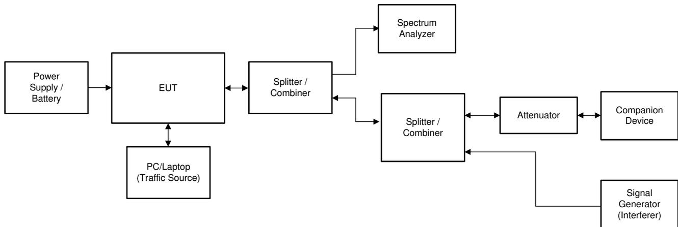
**Figure 3-1. Test Setup for Adaptivity Testing – EN 300 328**
