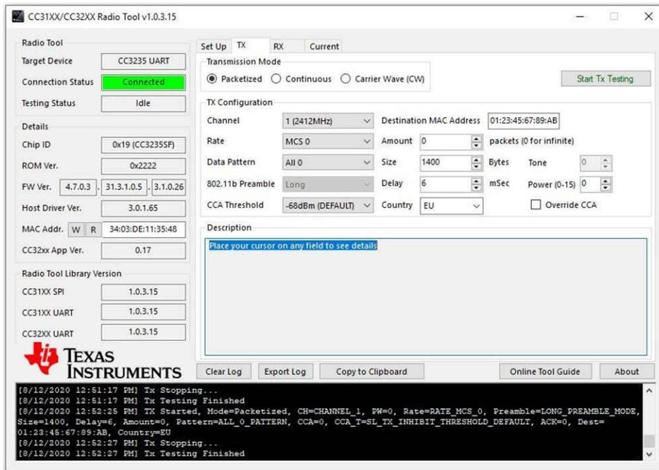
Figure 2-5. CC3235 – Configuration for 802.11n HT-20 Mode
