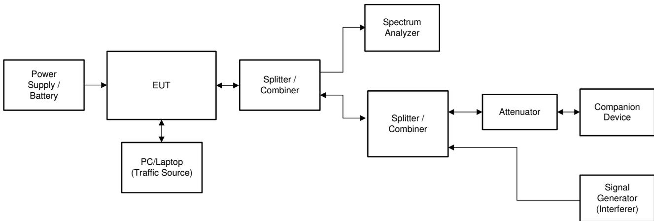
**Figure 4-2. Test Setup for Adaptivity – EN 301 893**
