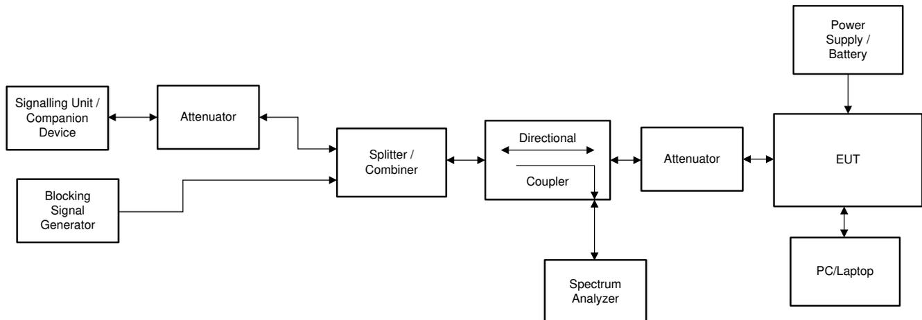
**Figure 4-1. Test Setup for Receiver Blocking – EN 301 893**
