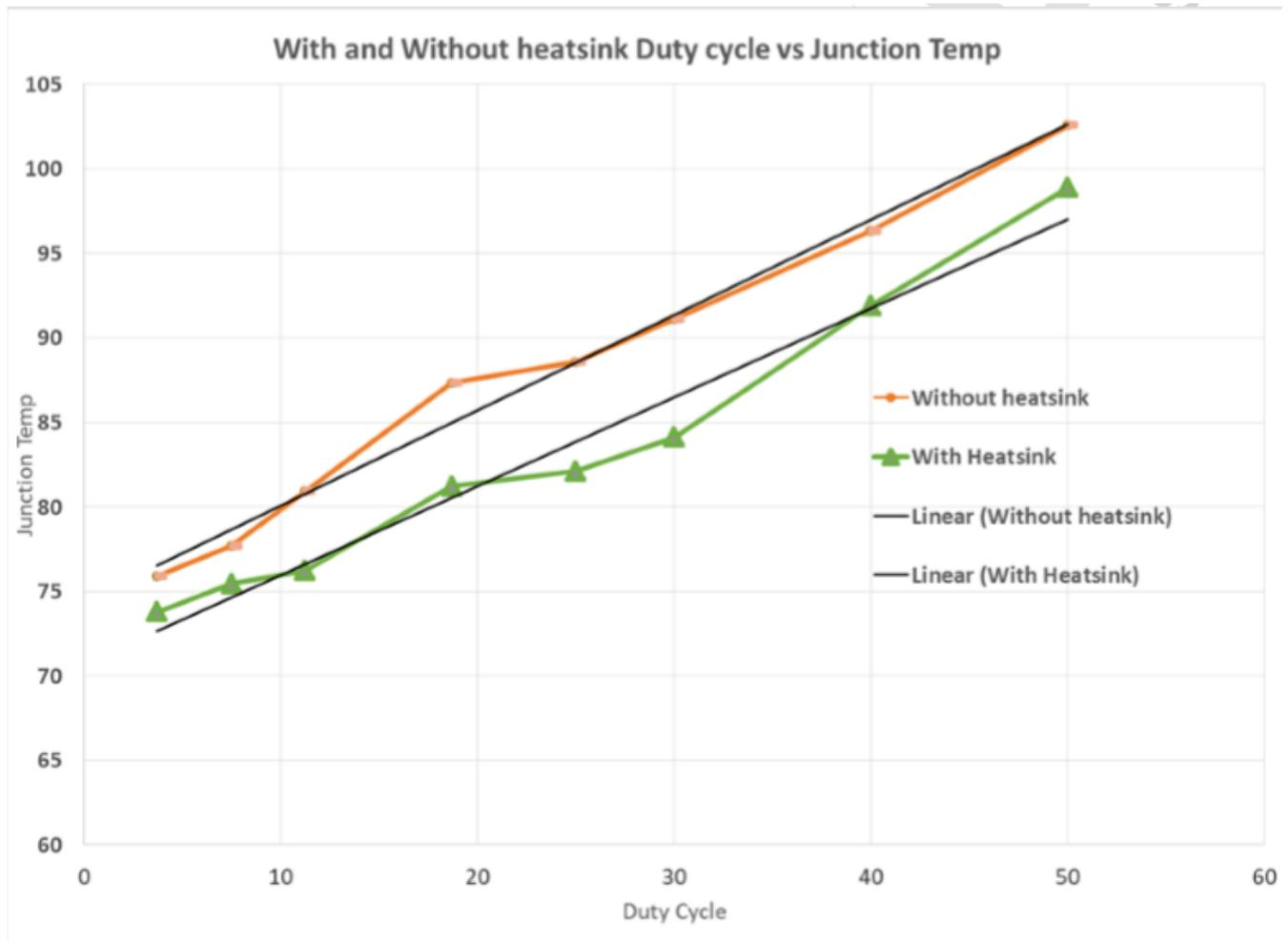
**Figure 11. Thermal Characteristics of mmWave AoP Sensor With and Without Sheet Metal-Based Heatsink**
