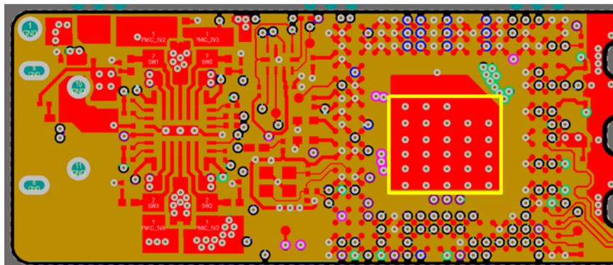
Figure 17. Top Side of the PCB Layout Around the Sensor and PMIC Regions
