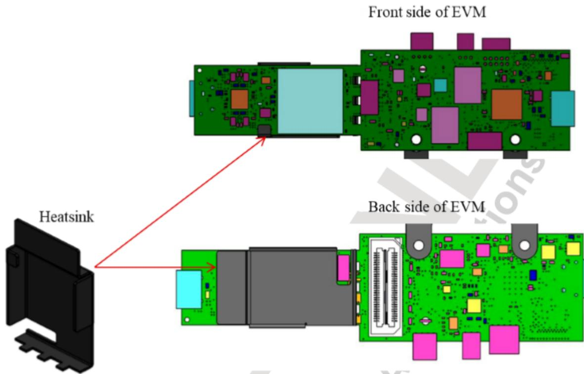
Figure 8. Sheet Metal Heat-Sink Used in the Form-Factor EVM
