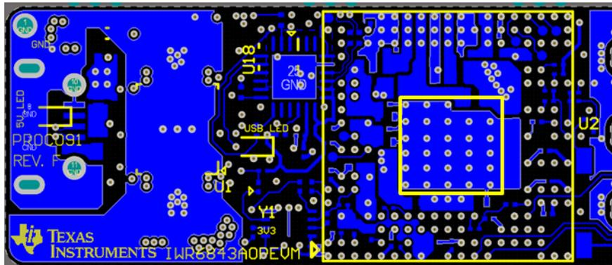
**Figure 18. Bottom Side of the PCB Layout Around the Sensor and PMIC Regions**
