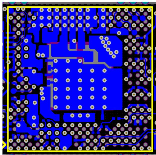
**Figure 20. Via Placement Under the BGA Bottom Side Layout Image**
