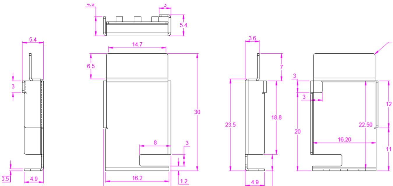
Figure 7. Sheet Metal Dimensional Details
