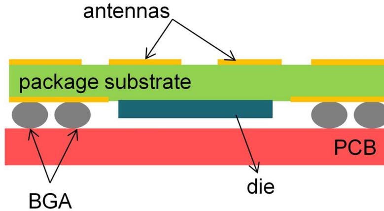
**Figure 1. Under-Mount Silicon Package on a PCB**
