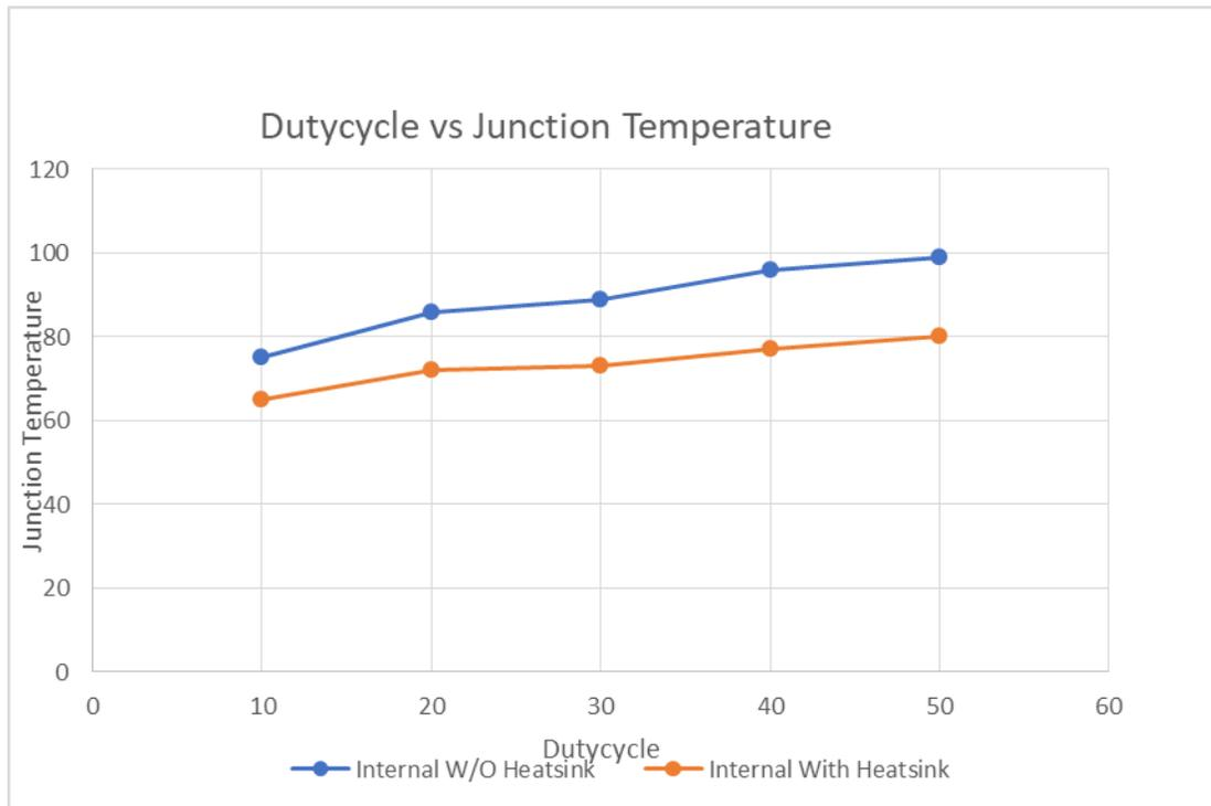
Figure 16. Thermal Characteristics of mmwave AoP Sensor With and Without FIN Metal-Based Heatsink
