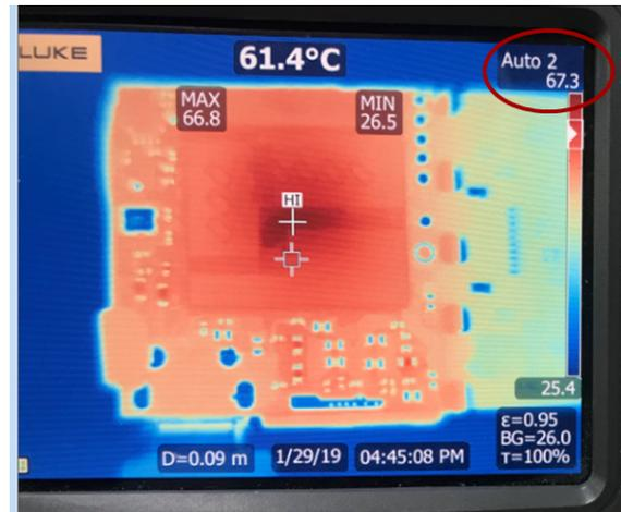
Figure 13. Thermal Imaging of the EVM (bottom side with heatsink mounted)
