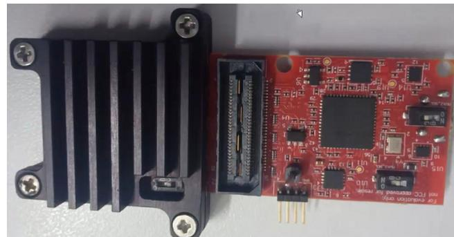
Figure 15. Bottom Side of the EVM With Heatsink With the FINS Mounted
