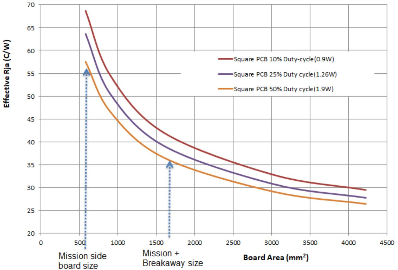
**Figure 4. Effective Thermal Resistance vs Board Size for Various Duty Cycles**
