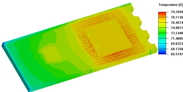
Figure 5. Thermal Simulation of Mission Side EVM With 10% Duty Cycle
