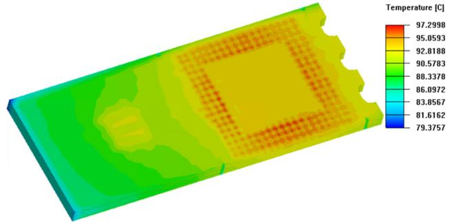
Figure 6. Thermal Simulation of Mission Side EVM With 25% Duty Cycle
