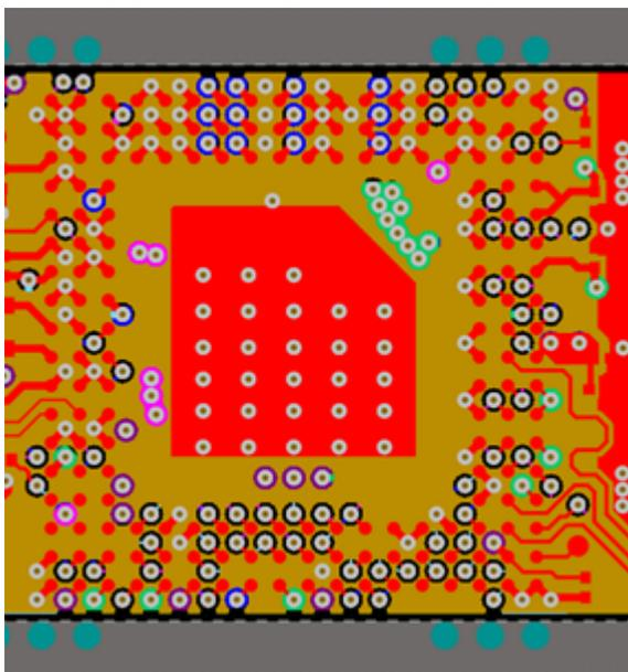
**Figure 19. Via Placement Under the BGA Top Side Layout Image**
