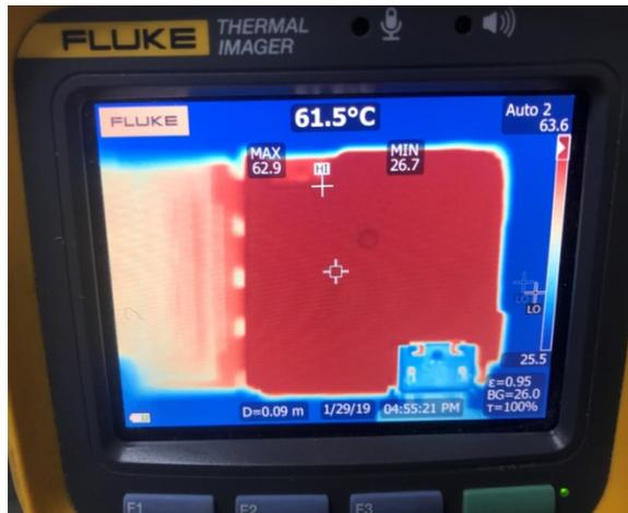
Figure 12. Thermal Imaging of the EVM (top side with heatsink mounted)
