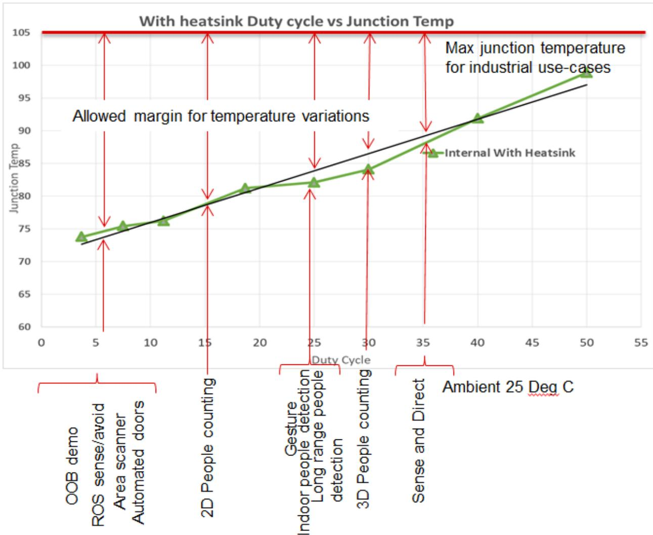
Figure 22. Thermal Characteristics of Various Demos Under Its Operating Conditions
