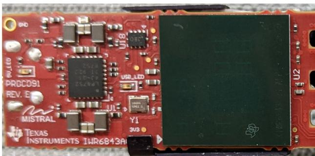
Figure 9. Top Side of the EVM With Heatsink Mounted
