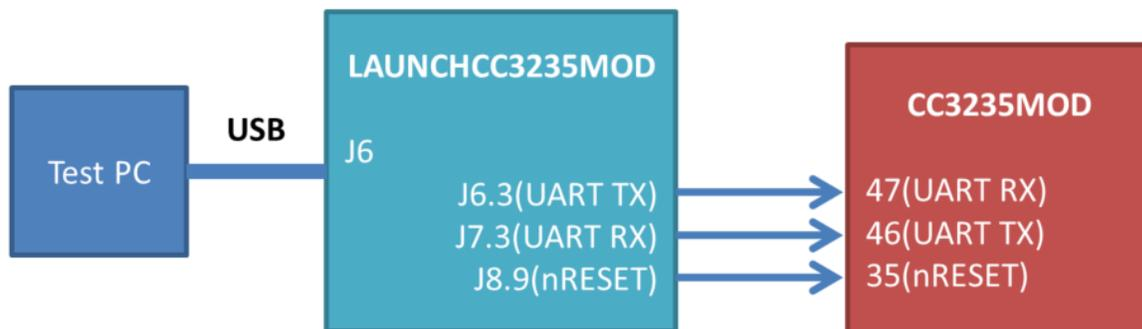
Figure 2. Connecting Through USB
