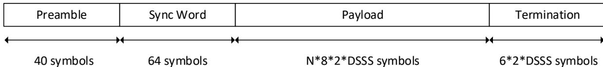
**Figure 5. Mode 1 Packet Structure**
