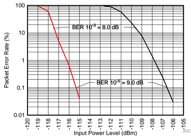
**Figure 4. Uncoded vs DSSS=4, K=7 PER (20-bytes) Performance**
