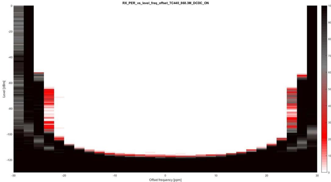
**Figure 7. Mode 2 Frequency Offset Performance (868 MHz, 5 kbps)**
