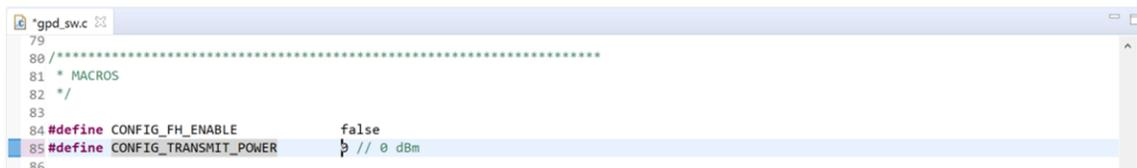
Figure 8. Setting TX Power Level for GPDs
