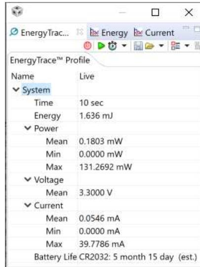
Figure 14. ZED EnergyTrace Measurement Profile
