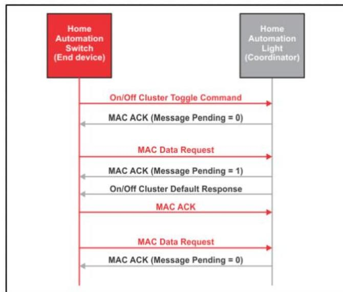
Figure 17. Message Sequence: End Device Switch Sends Toggle Command to a Coordinator Light
