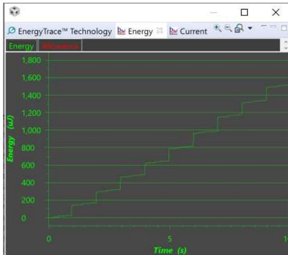
**Figure 16. ZED EnergyTrace Energy Measurement**
