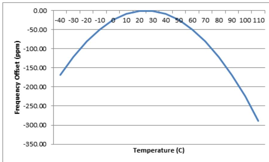
Figure 1. 32.768 Crystal Frequency Offset Over Temperature
