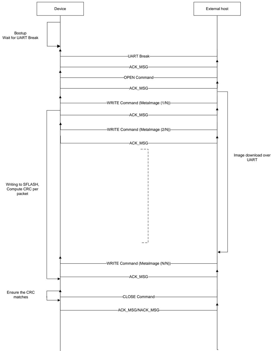
**Figure 9. Flashing Sequence**
