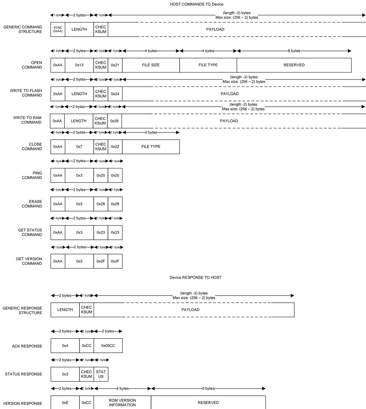
Figure 8. Host ← → IWR Device UART Communication
