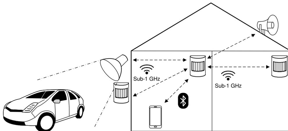
**Figure 3-3. Motion Detector System With Bluetooth low energy Connection**
