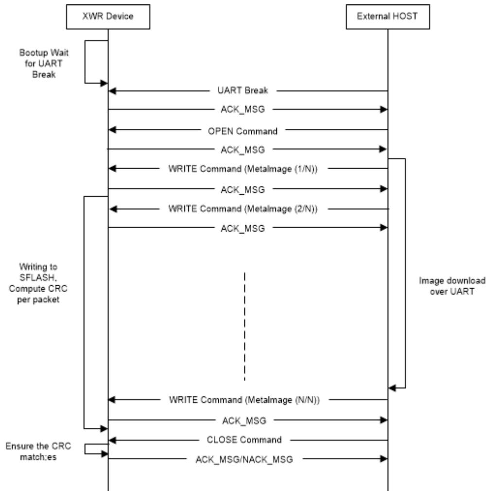
Figure 10. Flashing Sequence
