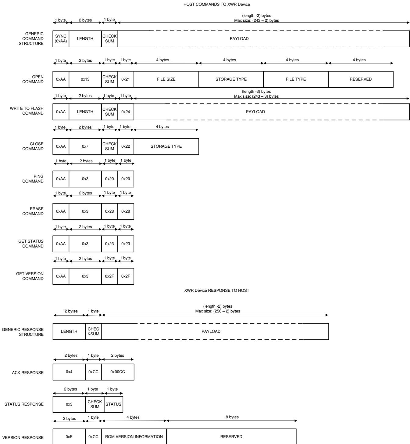
**Figure 9. HOST ↔ XWR Device UART Communication**
