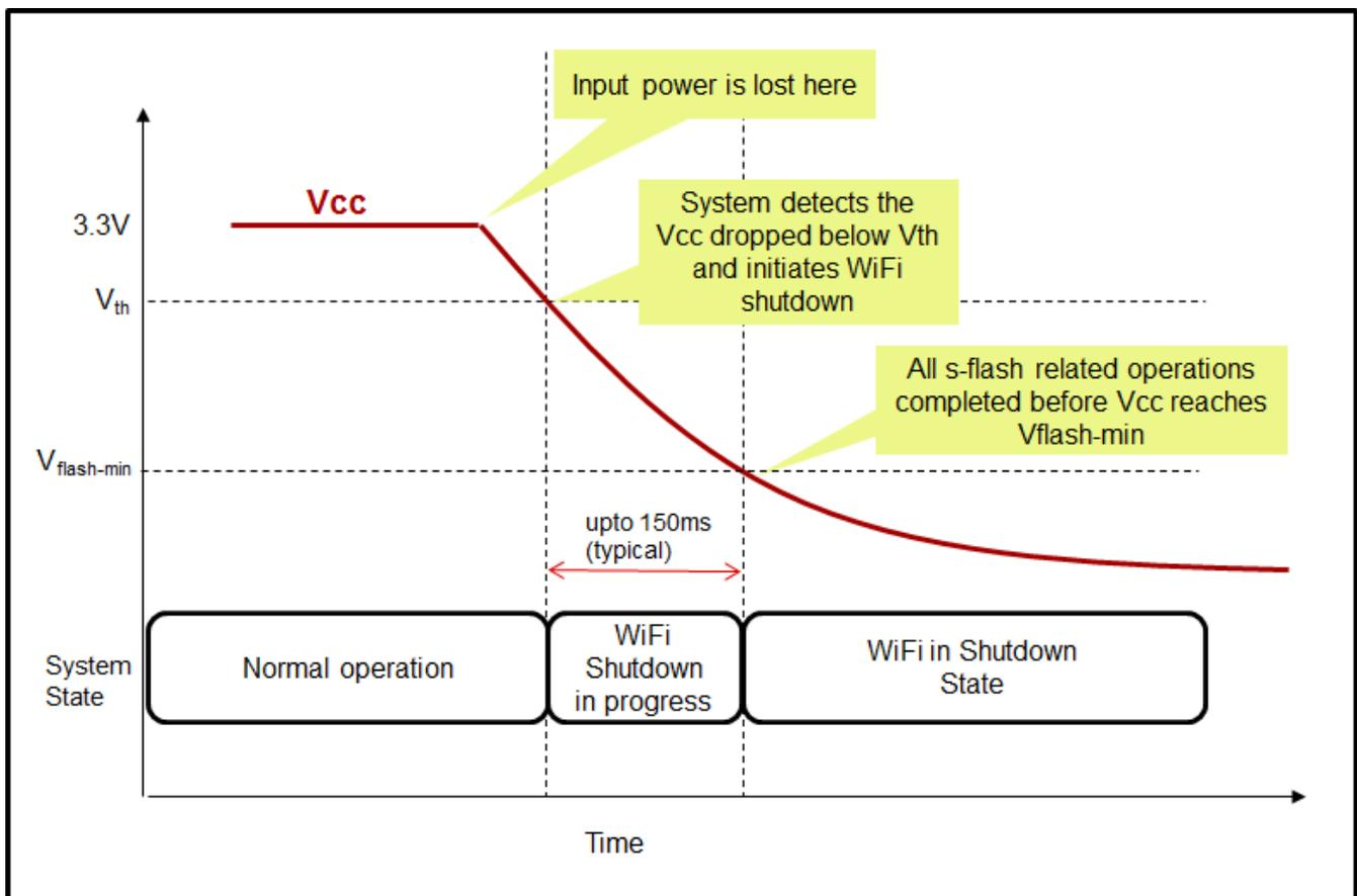
Figure 2. Sudden Power Off in Line-Powered Device
