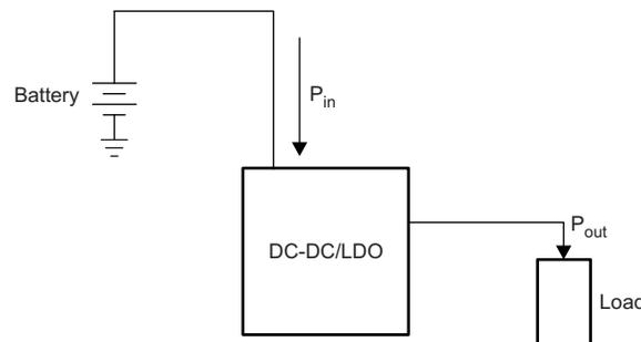
**Figure 5. Basic Regulator Configuration**
