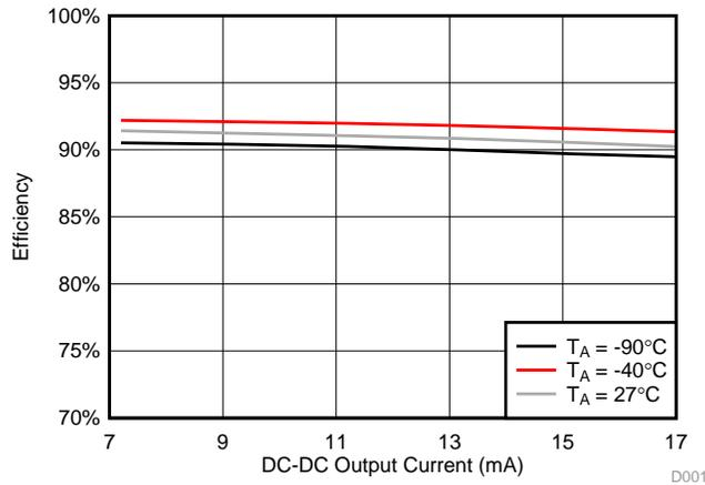
Figure 8. CC2640 Efficiency Across Temperature and Load Currents
