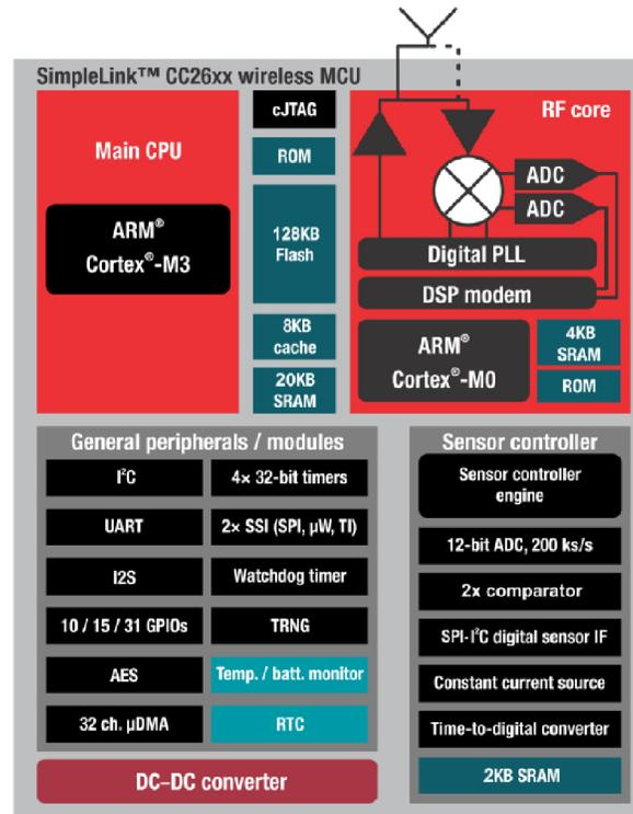
**Figure 1. CC2640 Block Diagram**
