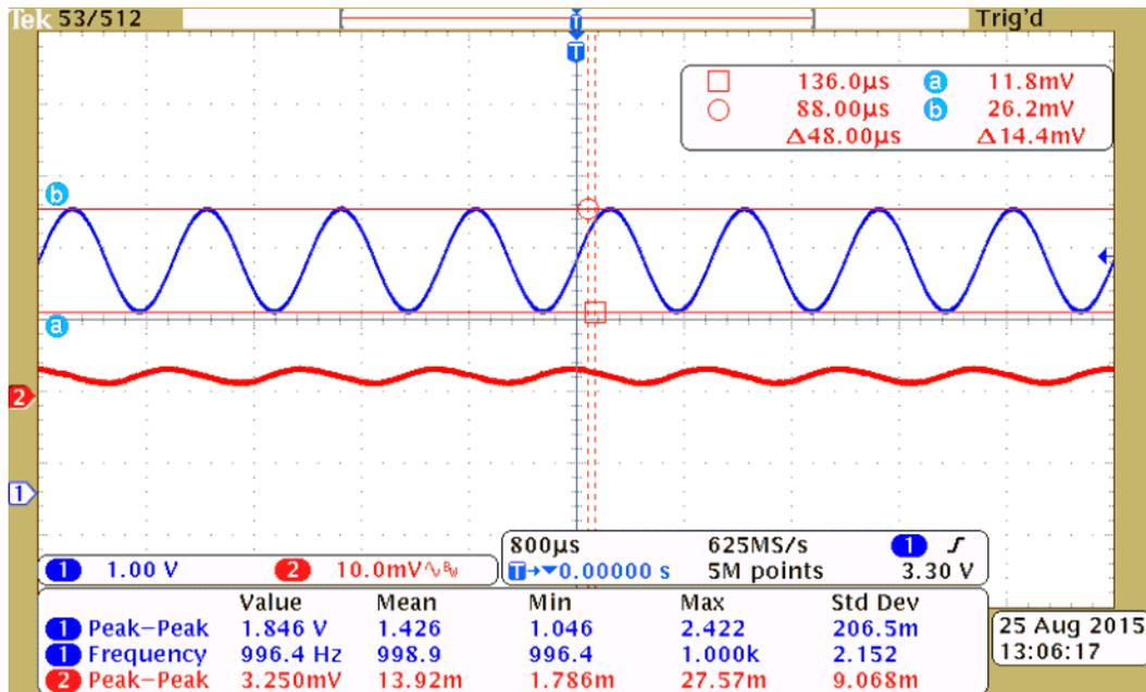
Figure 18. LDO PSRR Measurement Result, Frequency 1 kHz
