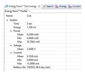
Figure 7-14. Average Current Consumption When Device Enters Standby
