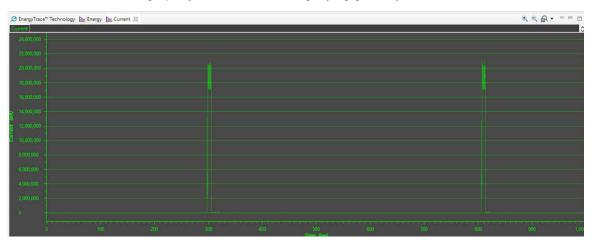
Figure 7-8. Current Profile for rfPacketTx (without modifications)
