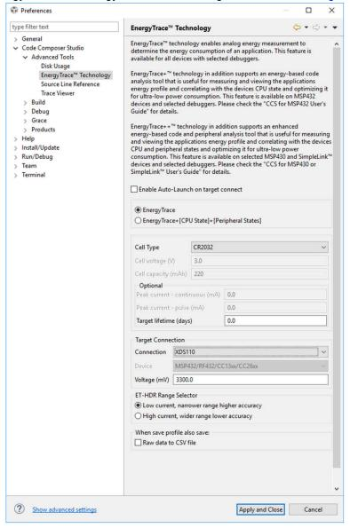
Figure 7-4. EnergyTrace Technology Configuration
