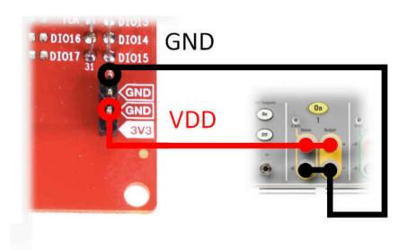
Figure 6-7. Connecting to the CC26x2r1 LaunchPad
