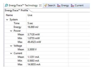
Figure 7-16. Average Current Consumption When Device Does not Enter Standby
