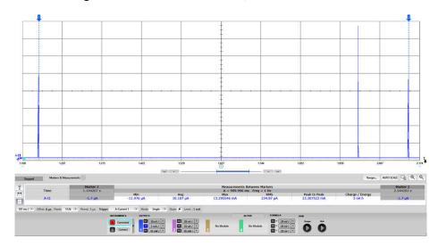
Figure 6-16. Average Current Consumption After Establishing a Connection
