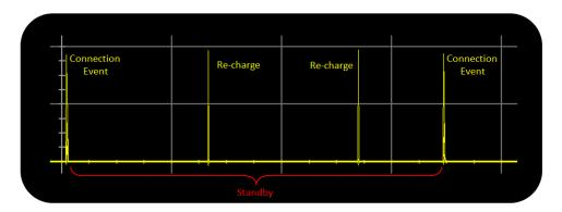
Figure 3-1. Current Consumption vs. Time During a Bluetooth Low Energy Connection
