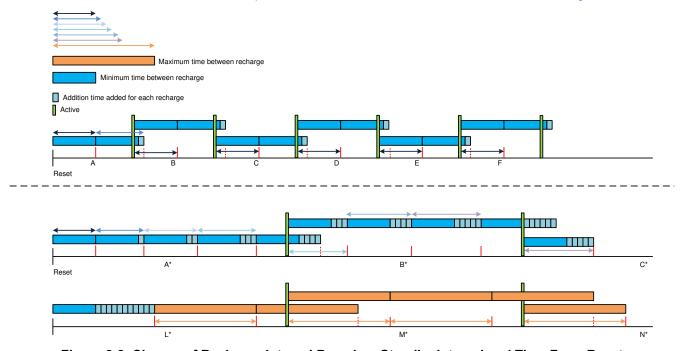
Figure 2-2. Change of Recharge Interval Based on Standby Interval and Time From Reset
