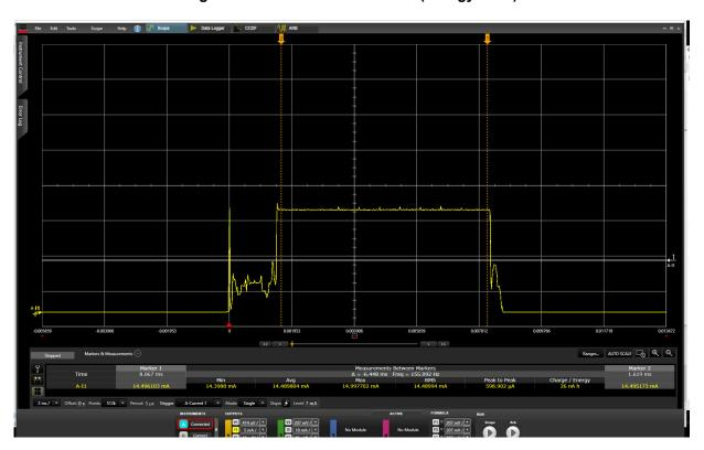
Figure 7-12. Current Profile of TX (DC Power Analyzer)
