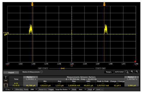
Figure 2-3. Measuring Standby Current During Advertisement (CC26x0)
