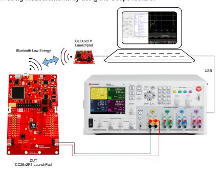
Figure 6-2. DUT Test Setup
