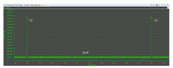
Figure 7-15. IDLE State Between Packets
