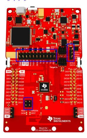
Figure 5-2. CC2652R LaunchPad Jumper Removal
