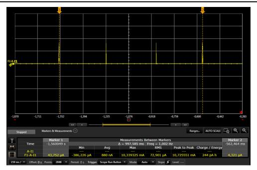
Figure 2-5. Measuring Standby Current During Connection (CC26x0)
