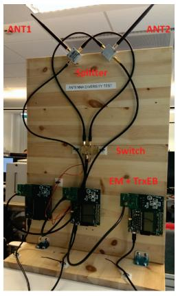
Figure 3. Antenna Diversity Test Board
