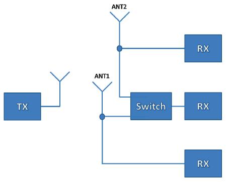
Figure 2. Block Diagram of Antenna Diversity Test Setup
