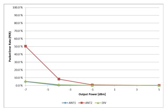
Figure 5. Packet Error Rate vs Output Power. Test Setup 4
