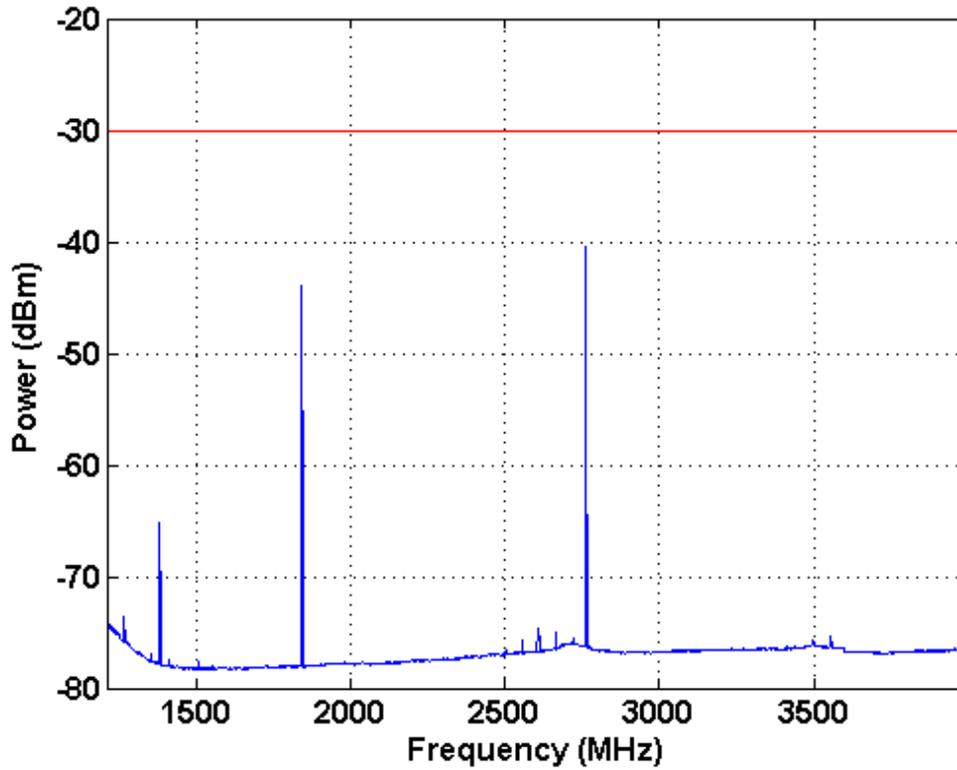
**Figure 10. Spurious Emission Above 1215 MHz**
