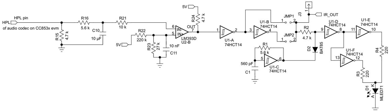
Figure 7. Processing of Received RC5 Remote Commands
