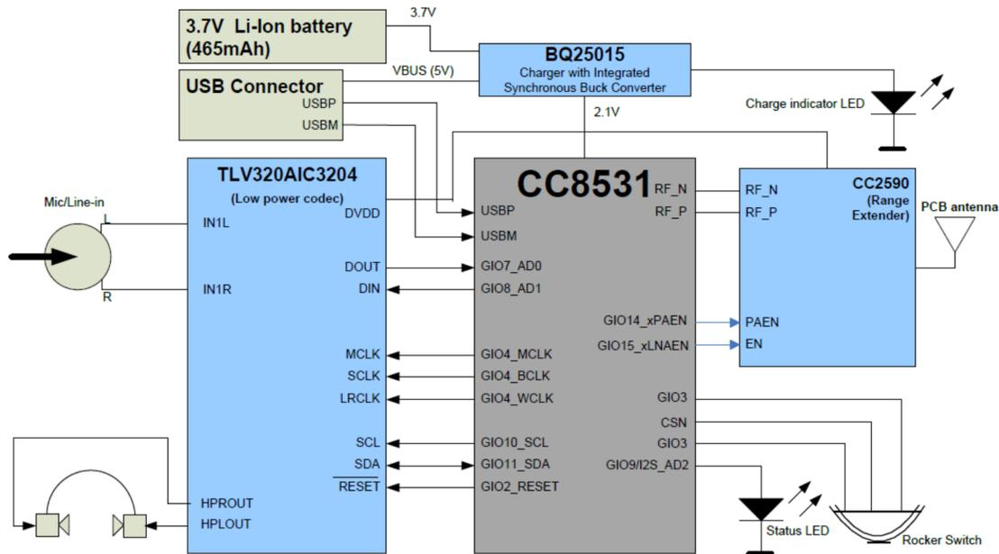
**Figure 1. Typical CC85xx and TLV320AIC3204 Application Schematic**
