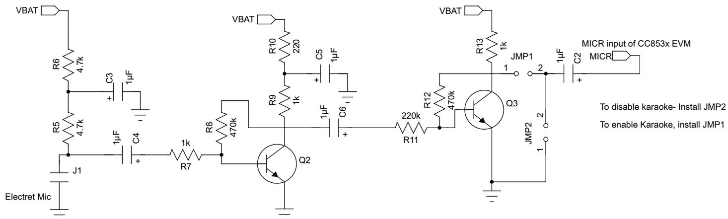
Figure 10. Remote-Side Schematics
