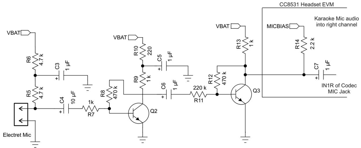
Figure 6. Karaoke MIC Audio into Right Channel
