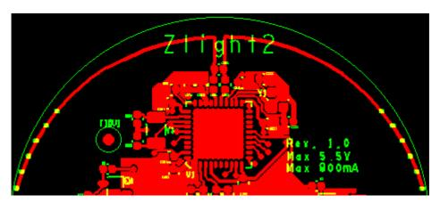
Figure 8. First Prototype Layout with Tuning Marks and Filtering Components
