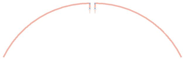
Figure 4. Curved Half Wave Dipole
