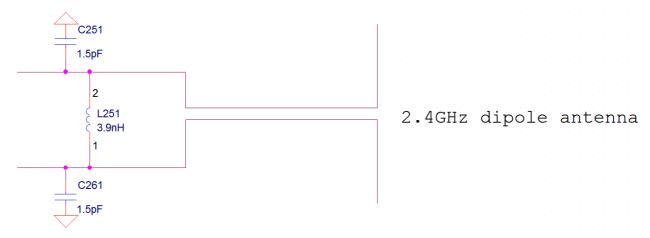
Figure 10. Parallel Resonant Circuit with Differential as well as Common Mode Rejection
