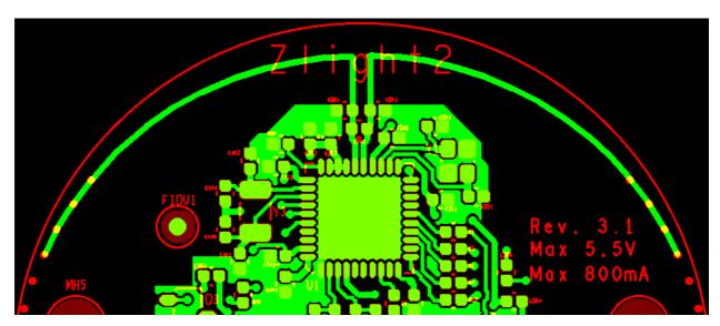
Figure 11. The Final Layout of the Antenna and Filtering Components
