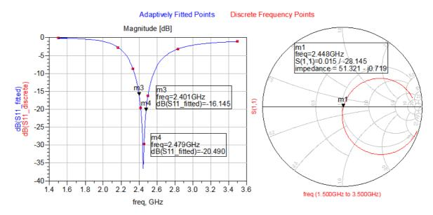
Figure 3. Simulated S11. Substrate: 800 um FR4
