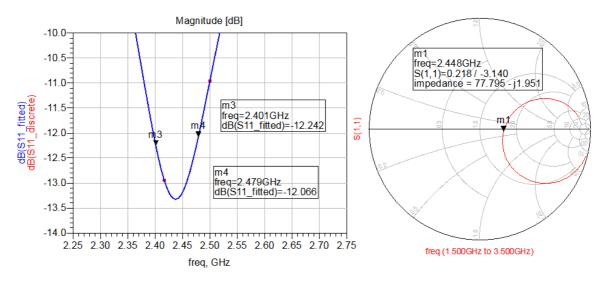
Figure 2. Simulated S11. Substrate: Free Space
