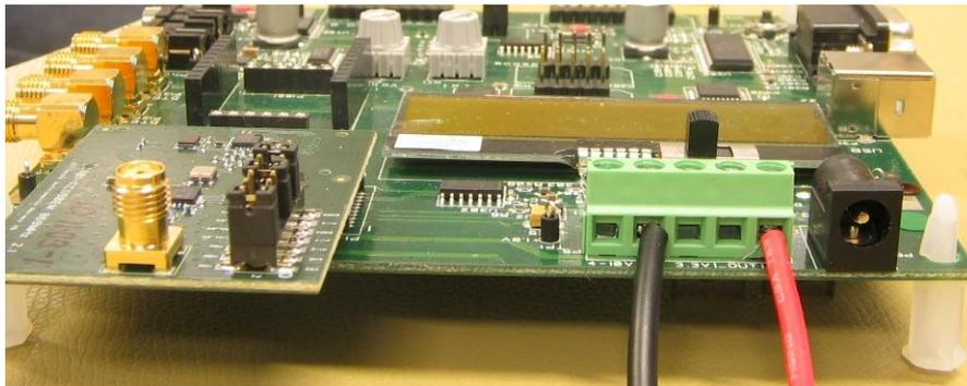
Figure 6.1. SmartRF04EB Connection
