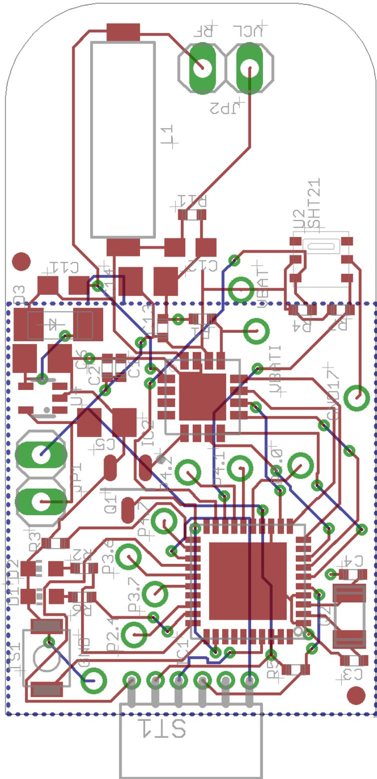
Figure 5. Eagle Layout of the Wireless Sensor
