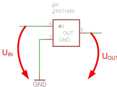
Figure 14.  $U_{IN}$  and  $U_{OUT}$  Voltage at DC/DC Regulator
