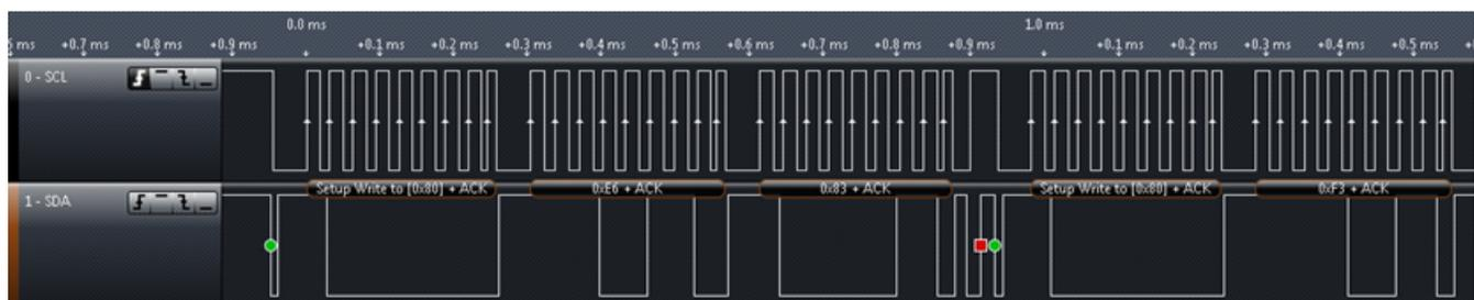
Figure 18. I2C Set Up and Start Temperature Measurement
