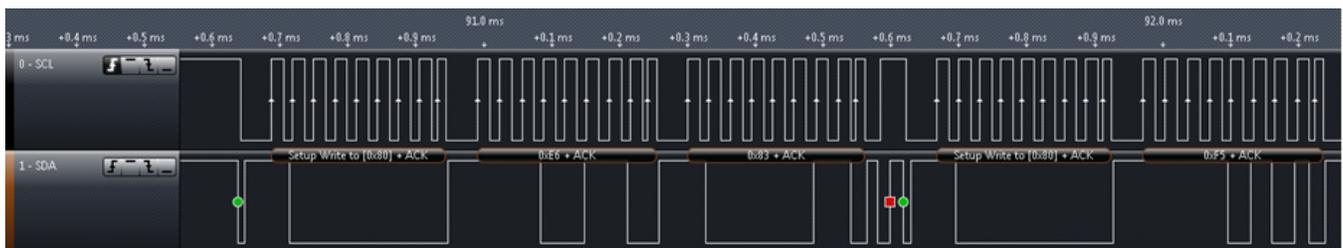
Figure 20. I2C Set Up and Start Humidity Measurement
