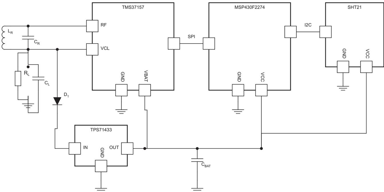
Figure 3. Principle Schematic of the Wireless Sensor
