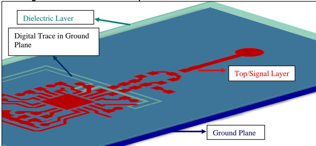
**Figure 6: Digital Lines directly below the RF path**
