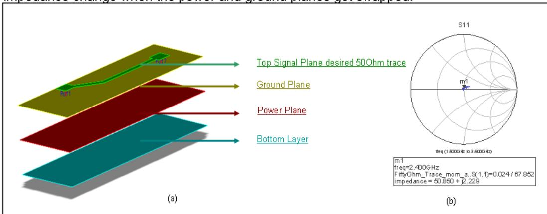
**Figure 8: Showing desired board stack up. Top plane with desired 50ohm trace followed by ground, power and then bottom layer. The simulated impedance of the trace is shown in (b) to be 50.85+j2.229 at 2.4GHz**
