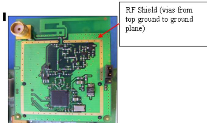
**Figure 4: Showing RF design with Grounded Via Shield**
