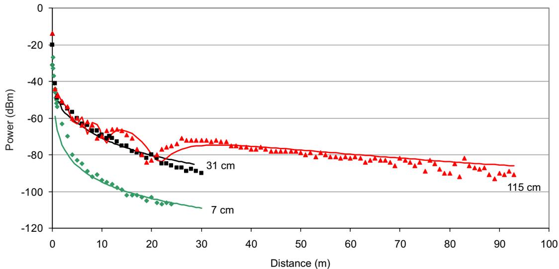
NOTE: Signal strengths with transmitter 7 cm, 31 cm, and 115 cm above ground.
