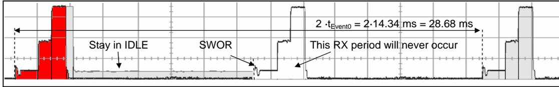
**Figure 7. Current Consumption vs. Time (Avoiding Time Shift)**
