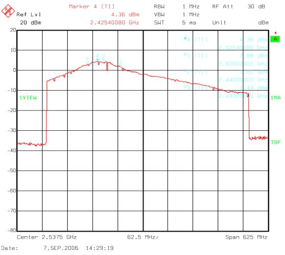
Figure 11: Bandwidth of folded dipole antenna.
