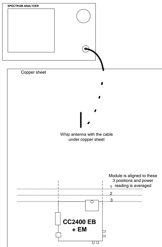
**Figure 5: Tuning Setup**
