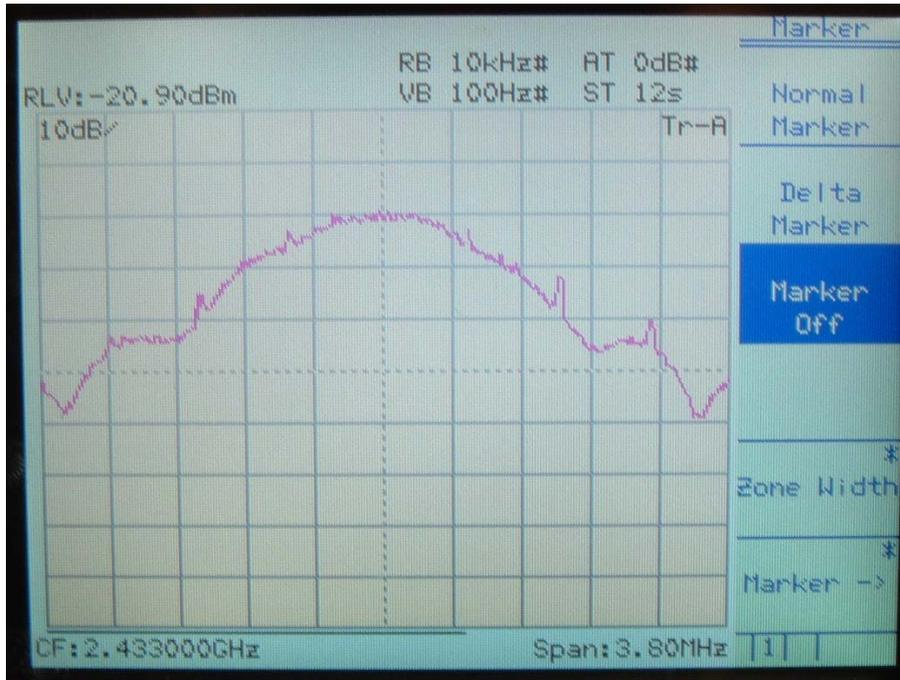
**Figure 4: Example of Poor Spectrum. Antenna Removed from EM**
