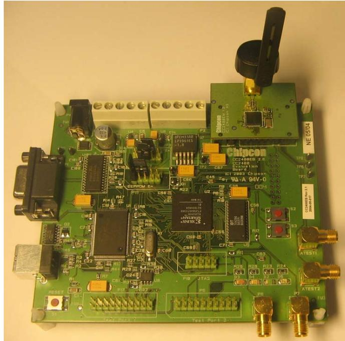
Figure 6: EB with CC2400EM with Whip Antenna
