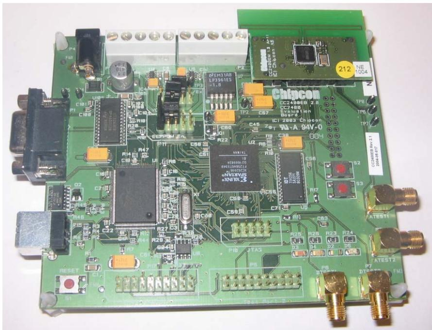
Figure 7: EB with CC2400EM with Folded Dipole Antenna
