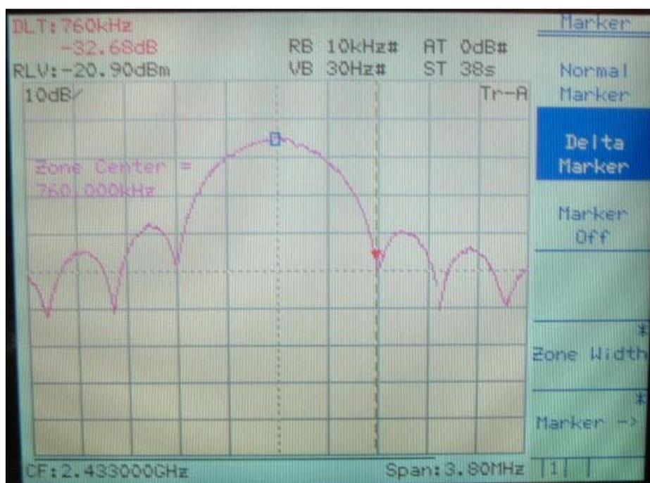
Figure 3: Reference Spectrum for CC2400 at 1 Mbps
