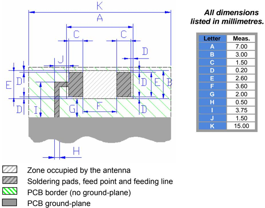
**Figure 4: Footprint Details on the CC2400 USB Dongle**
