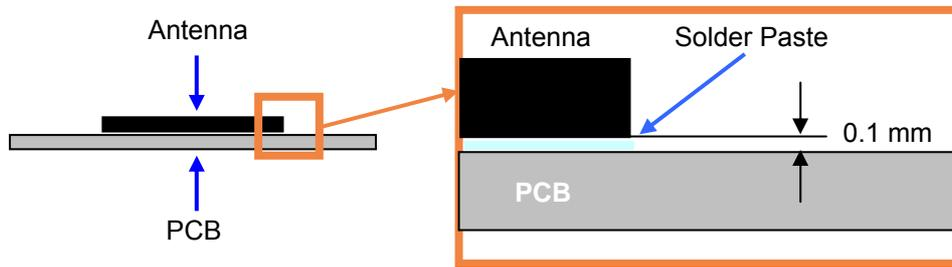
**Figure 7: Soldering Details**
