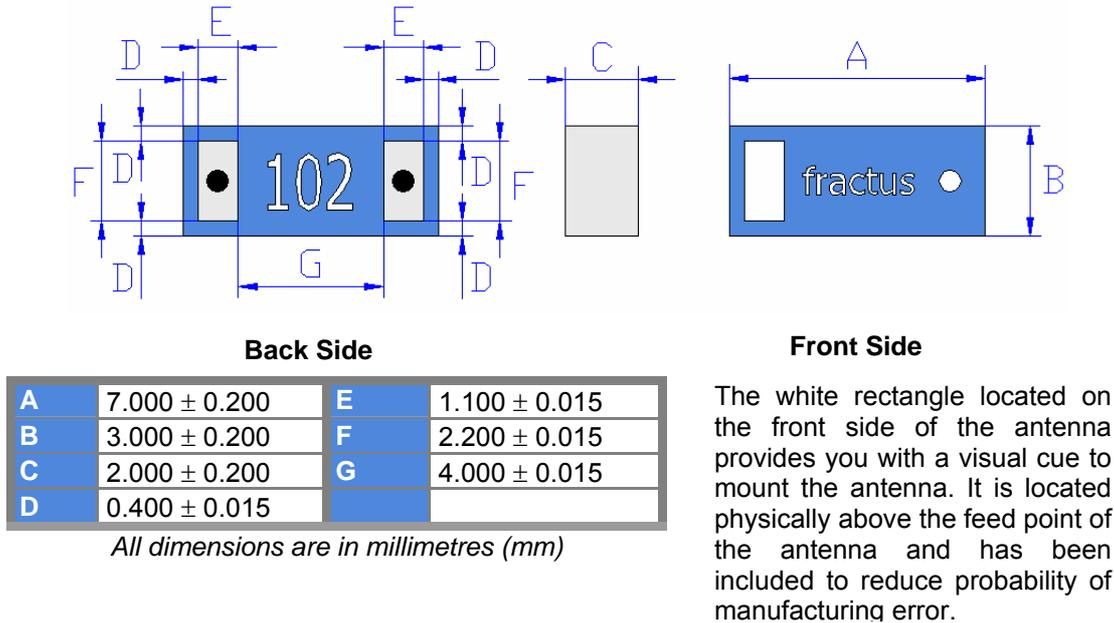
Figure 5: Antenna Dimensions and Tolerances
