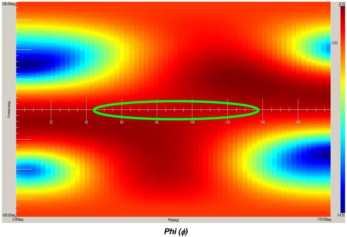
Figure 3: Gain [dBi] Projected in 2D Plot from a 3D Measurement
